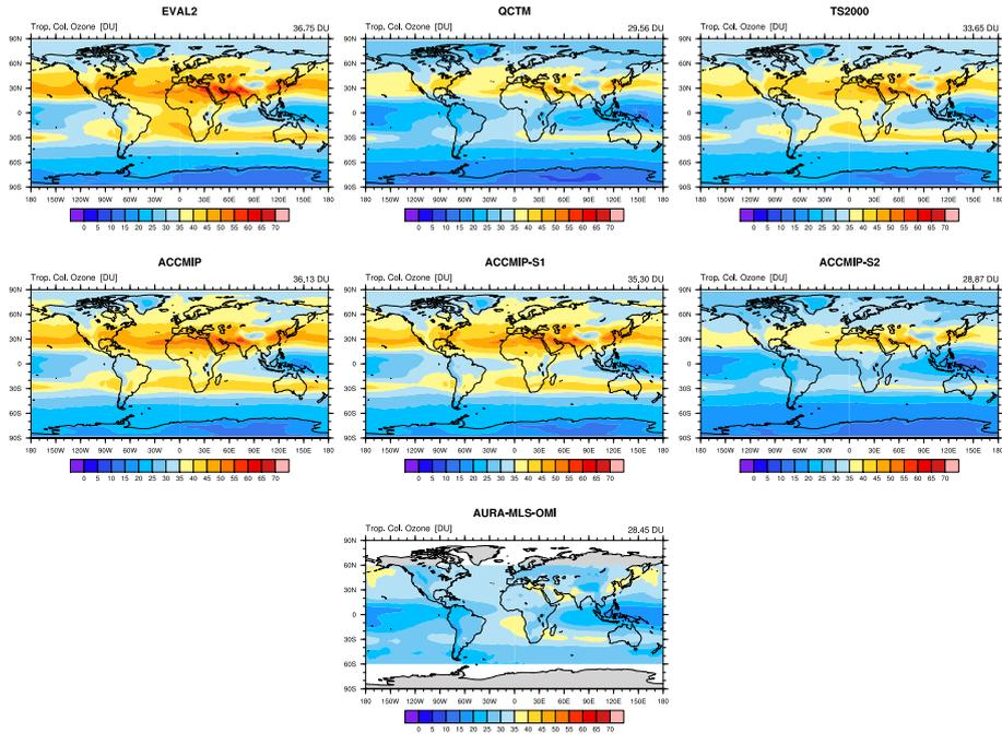
**Figure 13.** Tropospheric column ozone in the EMAC simulations compared to MLS/OMI observations. The values on top of each panel show the global (area-weighted) average, calculated after regridding the data to the horizontal grid of the model and ignoring the grid cells without available observational data.
