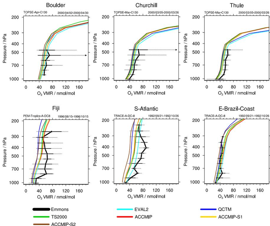
**Figure 16.** Ozone vertical profile climatology from selected aircraft campaign observations by Emmons et al. (2000) and corresponding simulated values by the EMAC simulations. Profiles represent mean values. The EMAC simulations are averaged over the same regions and time of year as the observations, but for different years. Solid whiskers indicate  $\pm 1$  standard deviation and dotted whiskers show minimum and maximum, both for the observational data.
