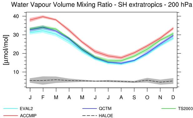
**Figure 3.** Annual cycle of water vapour climatology at 200 hPa averaged over the SH extratropics ( $20\text{--}90^\circ\text{S}$ ) for the EMAC simulations in comparison to HALOE data. Shaded area indicates the  $\pm 1\sigma$  interannual variability.
