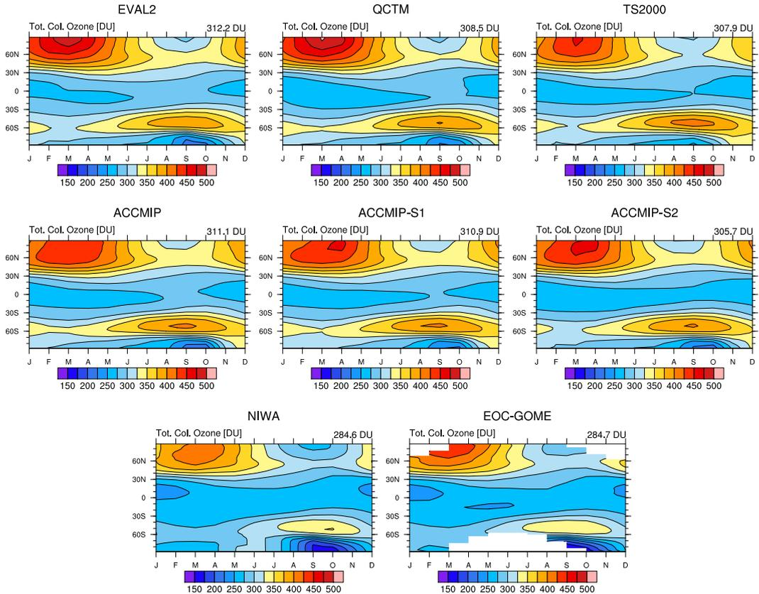
**Figure 10.** Total column ozone climatology for the EMAC simulations compared to the NIWA combined total column ozone database and GOME data. The values on top of each panel show the global (area-weighted) average, calculated after regriding the data to the horizontal grid of the model and ignoring the grid cells without available observational data in the GOME dataset.
