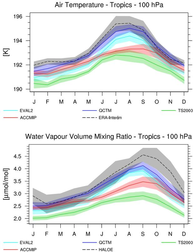
**Figure 4.** Annual cycle of temperature (top) and water vapour (bottom) climatology at 100 hPa averaged over the tropics ( $20^{\circ}\text{N}$ – $20^{\circ}\text{S}$ ) for the EMAC simulations, in comparison to ERA-Interim re-analysis and HALOE data, respectively. Shaded areas indicate the  $\pm 1\sigma$  interannual variability.
