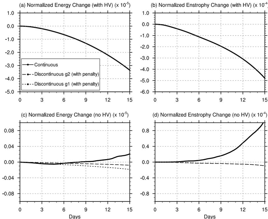
**Figure 7.** Normalized total energy and potential enstrophy change for the zonal flow over an isolated mountain test with  $n_e = 16$  and  $n_p = 4$  over a 15 day simulation. In **(a)** all simulations show roughly equivalent energy and enstrophy loss and so all lines are coincident. In **(c)** and **(d)** the simulation with continuous elements is beginning to experience instability, leading to total energy and enstrophy growth after approximately 6 days simulation time.
