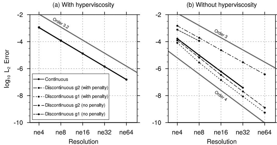
**Figure 5.**  $L_2$  errors for geostrophically balanced flow on the cubed-sphere at various resolutions with  $n_p = 4$  over a 5 day integration period. In **(a)** errors due to hyperviscosity dominate and so all simulations have approximately equal error leading to coincident lines. In **(b)** unstable simulations have been removed.
