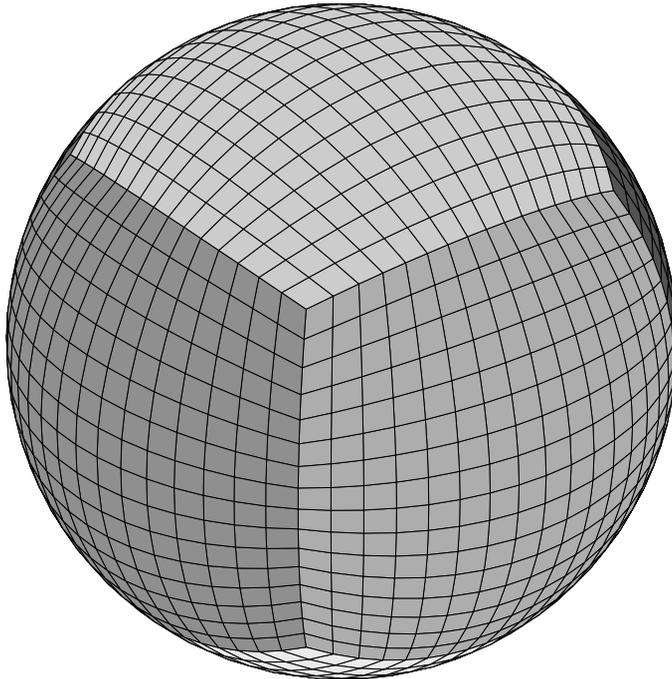
**Figure 1.** A 3-D view of the cubed-sphere grid shown here with  $n_e = 16$ . Cubed sphere faces are individually shaded.
