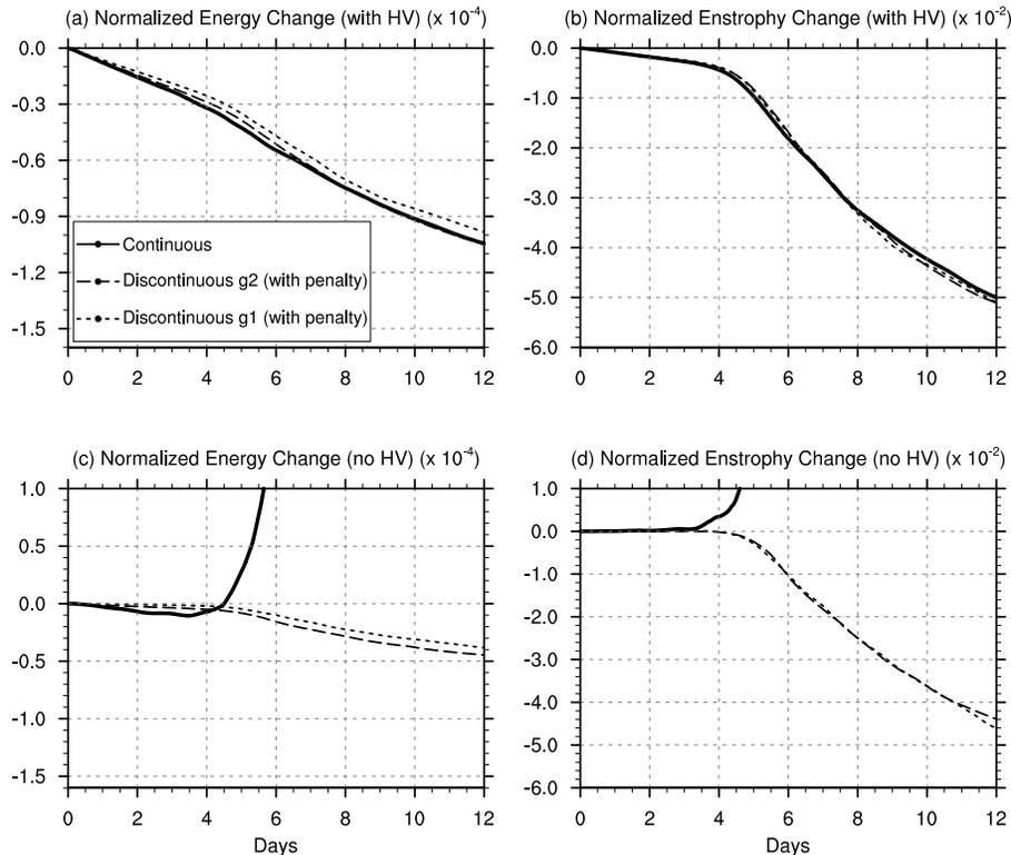
**Figure 9.** Normalized total energy and enstrophy change for the barotropic instability test with  $n_e = 16$  and  $n_p = 4$  over a 12 day simulation. In (c) and (d) the continuous element simulation fails after approximately 6 days, leading to unbounded growth in energy and enstrophy. The time step used for these runs was (a, d)  $\Delta t = 300$  s, (b, e)  $\Delta t = 150$  s and (c, f)  $\Delta t = 75$  s. Discontinuous penalization was used for both discontinuous schemes.
