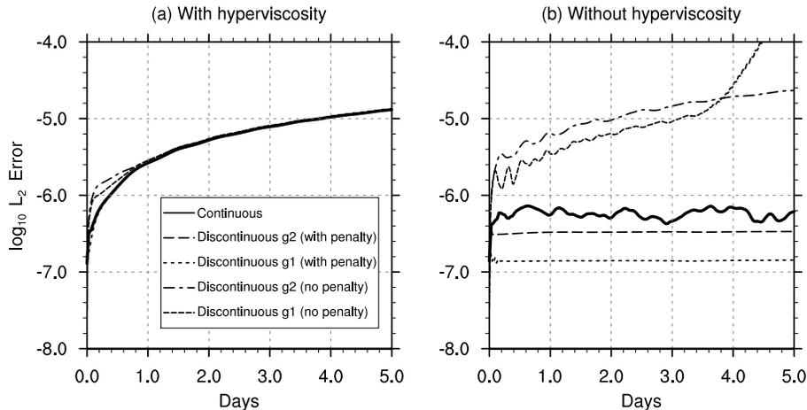
**Figure 4.**  $L_2$  error time series for geostrophically balanced flow on the cubed-sphere for  $n_e = 16$  and  $n_p = 4$  over a 5 day integration period for all continuous and discontinuous schemes.
