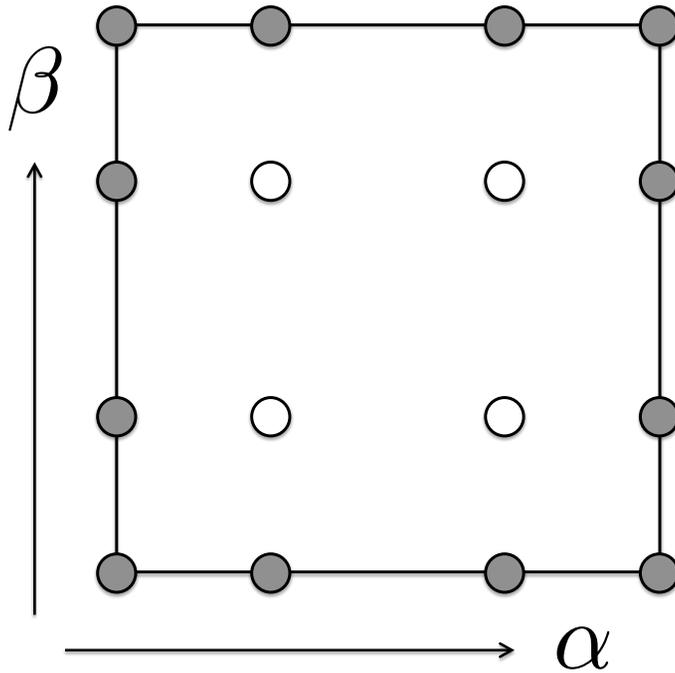
**Figure 2.** A depiction of the nodal grid for a reference element on GLL nodes for  $n_p = 4$ . Boundary nodes, which are connected to neighboring elements, are shaded.
