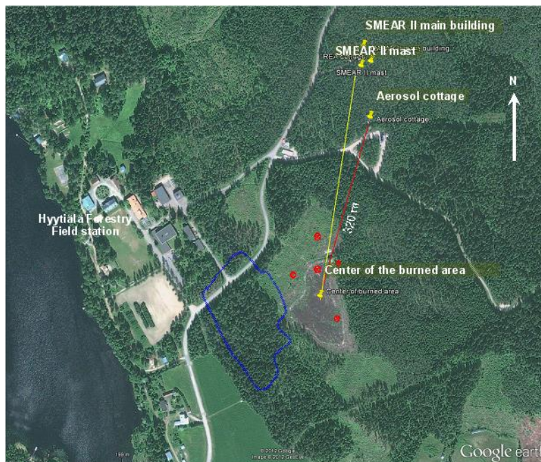
Fig. 1. Location of the burned area (in grey), the SMEAR II main building, mast, and aerosol cottage (yellow pins), and the meteorological measurements within and around the burning area (red dots). The distance from the centre of the burned area to the aerosol cottage is 320 m. The blue line encircles a non-burned reference area. This Google Earth satellite image was taken on 4 July 2010, approximately a year after the burn.
