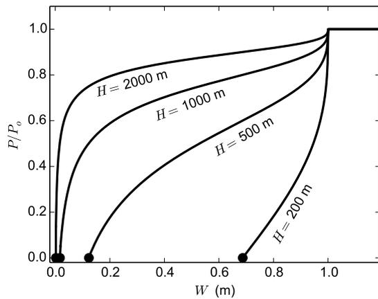
**Fig. A12.** The graph of  $P(W)$  defined by (A3) also depends on overburden pressure  $P_o = \rho_i g H$ . We fix, shown using  $|v_b| = 100$  m/a and  $W_r = 1$  m and consider four cases of uniform thickness  $H$ .
