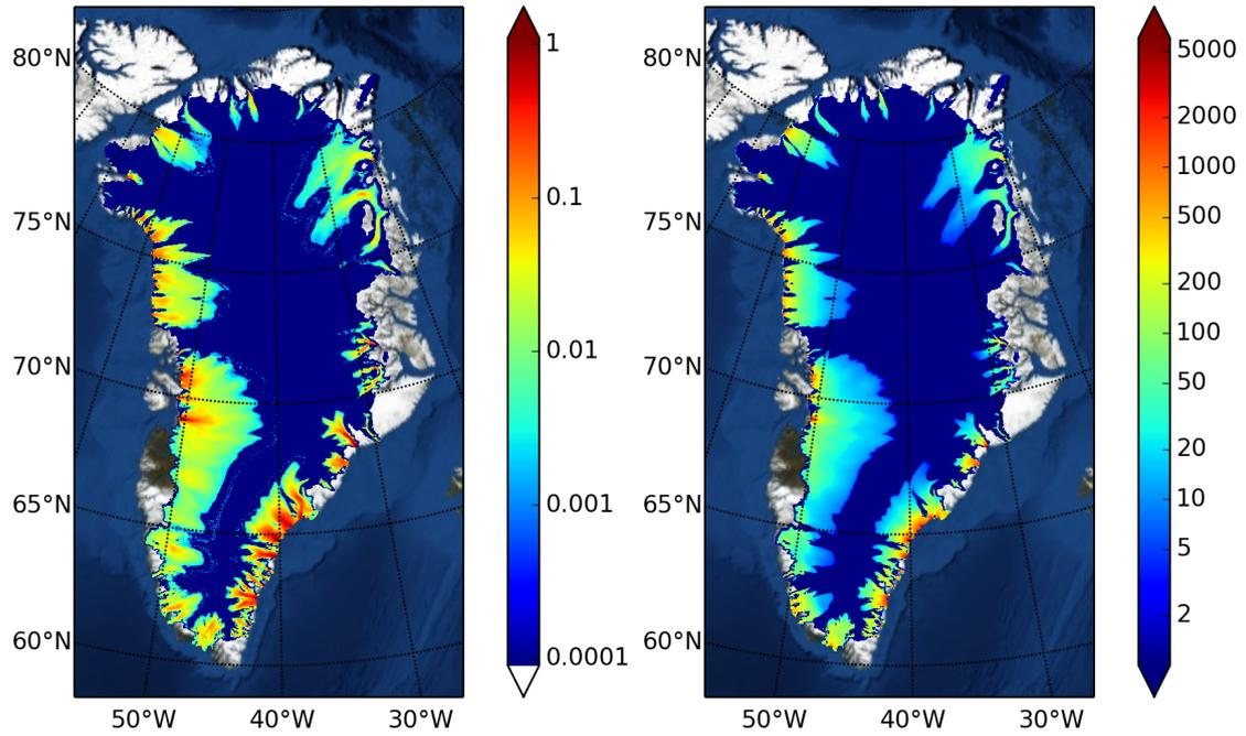
**Fig. A6.** The inputs to the hydrology model are the modeled basal melt rate  $m/\rho_w$  (left;  $\text{m a}^{-1}$ ) and sliding speed  $|v_b|$  (right;  $\text{m a}^{-1}$ ) from the spun-up [modelstate](#).
