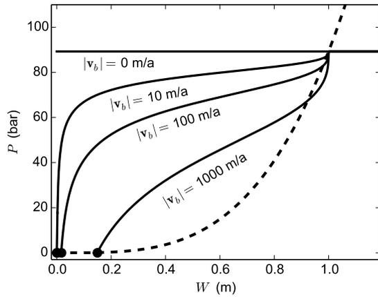
**Fig. A11.** The steady state function  $P(W)$  defined by equation (A3) depends on the sliding speed  $|v_b|$ . Four cases are shown. All use, using  $W_r = 1$  m and a uniform ice thickness of  $H = 1000$  m (solid curves). Values of  $W_c$  are indicated by black dots at  $P = 0$ . Relation For comparison, Flowers and Clarke (2002a) relation (28) (dashed black) is shown with  $W_{crit} = 1$  m for comparison (dashed black).
