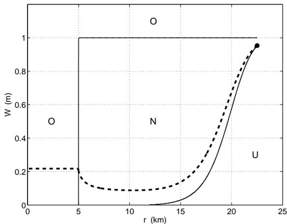
**Fig. A2.** An exact radial, steady solution for water thickness  $W(r)$  (dashed). In  $r$ -versus- $W$  space the overpressure (O), normal pressure (N), and underpressure (U) regions (solid curves) are determined by ice geometry and sliding velocity (solid curves; see text), because this is steady state.
