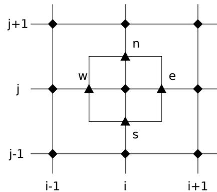
**Fig. A4.** Numerical schemes (44) and (49) use a grid-point-centered cell. Velocities, diffusivities, and fluxes are evaluated at staggered grid locations (triangles at centers of cell edges) denoted by compass notation  $e, w, n, s$ . State functions  $W, P, W, P$  are located at regular grid points (diamonds).
