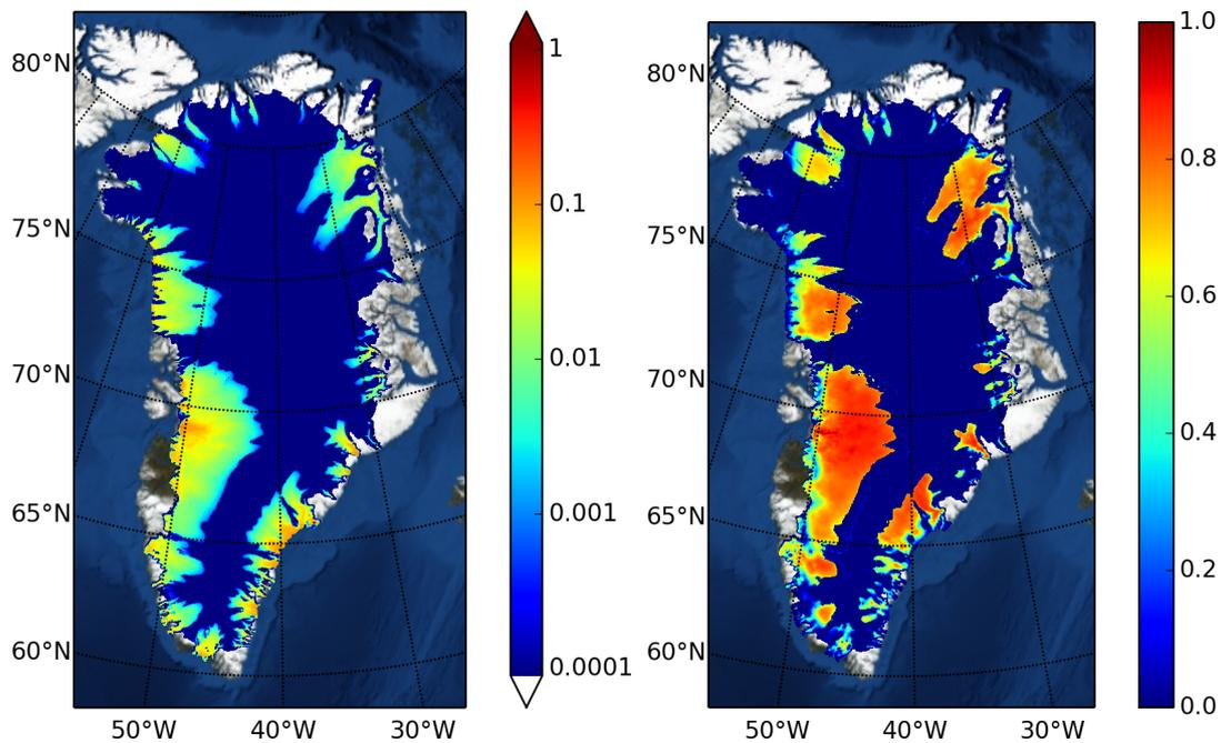
**Fig. A9.** Outputs from the distributed hydrology model include the modelled transportable water layer thickness  $W$  (left; m), and the modelled transportable water layer pressure  $P$ , shown relative to overburden pressure  $P/P_o$  (i.e.  $P/P_e$ ; right).
