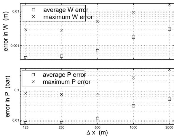
**Fig. A5.** Average water thickness error  $|W - W_{exact}|$  decays as  $O(\Delta x^{0.91})$ , and average pressure error  $|P - P_{exact}|$  decays as  $O(\Delta x^{0.92})$ , for grids with spacing  $250 \leq \Delta x = \Delta y \leq 2000$  m.
