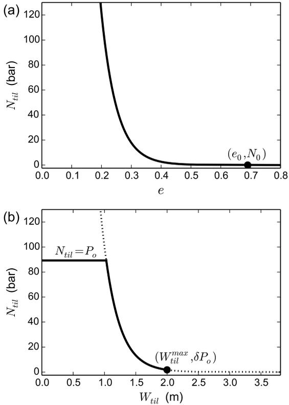
**Fig. A1.** (a) Equation (19) determines the effective pressure  $N_{til}$  as a function of the void ratio  $e$ , as shown here. Reference values of  $e_0$  and  $N_0$  are indicated. (b) The same curve, but with  $N_{til}$  as a function of  $W_{til}$ , and bounded with bounds above by overburden pressure  $P_o$  and below by a fixed fraction  $\delta$  of  $P_o$  (the solid curve) is used in our model. The case shown is for 1000 meters ice thickness.
