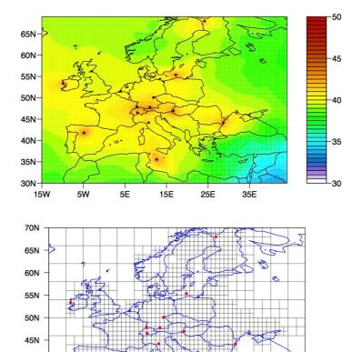
Figure 2. Total emission sensitivity for 2011 in units of  $log(s m^{-3} kg^{-1})$  (a) and the variable resolution grid used in the inversion (b). The points indicate the positions of the observation sites.
