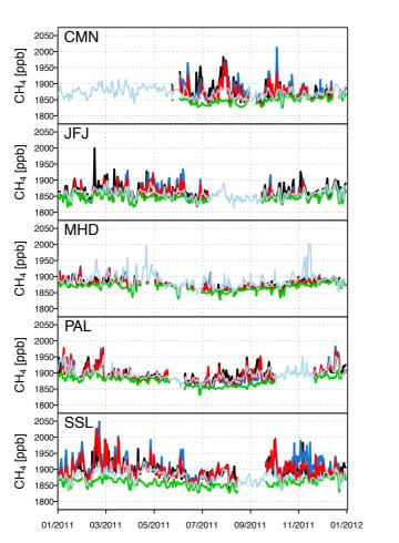
**Figure 3.**  $CH_4$  mole fractions (ppb) as observed (black) and simulated from the prior (blue) and posterior models (red). Also shown is the background  $CH_4$  mole fraction (green) and  $CH_4$  calculated by the TM5 Eulerian model (light blue).
