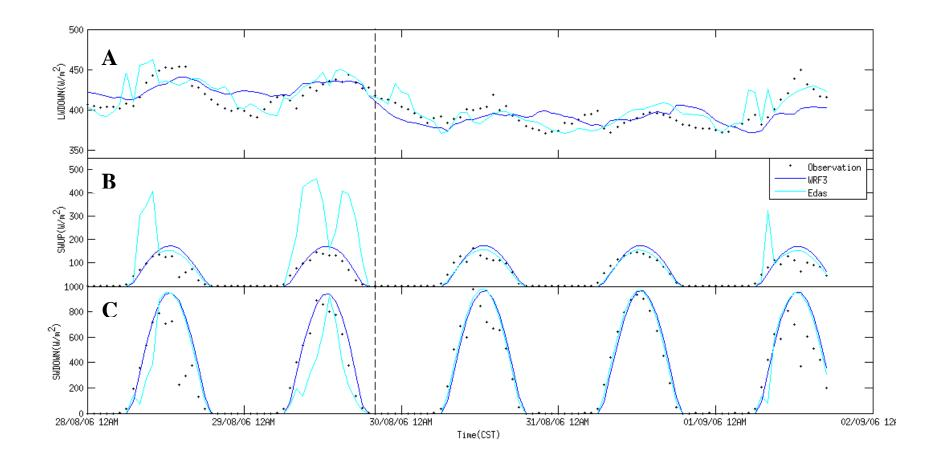
Figure. 4. Time series for incoming longwave (A), outgoing shortwave (B), and incoming shortwave (C) radiation for observations (dots) and for
