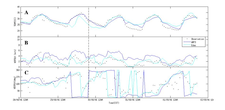
Figure. 3. Time series of temperature (A), wind speed (B), and wind direction (C) for observations (dots) and for the WRF (blue) and MM5 with
