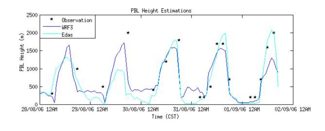
801 Figure. 7. Comparison of observed and simulated PBL height for the study period. The WRF
