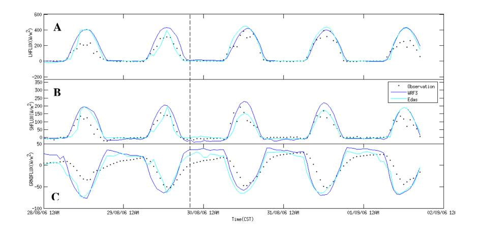
Figure. 5. Time series for latent heat (A), sensible (B), and ground (C) flux for observations (dots) and for the WRF (blue) and MM5 with EDAS
