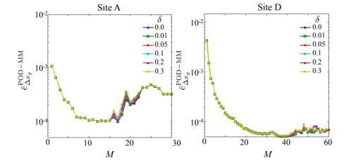
**Fig. 18.** The variation of  $\overline{e}_{\Delta x_a}^{\text{POD-MM}}$ with respect to M for different  $\delta$  and for  $\Delta x_q = 8 \,\mathrm{m}; \ \delta = 0$  is the reference case where there is no bias. Results are shown for sites A and D for year 2006.
