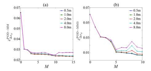
**Fig. 15.** The errors **(a)**  $\overline{e}_{\Delta x_g}^{\text{POD-MM}}$  and **(b)**  $\overline{e}_{\Delta x_g}^{\text{POD-MM3}}$  vs. M for different  $\Delta x_g$  at site A. The means are taken over 1998, 1999, 2000, 2002, and 2006.
