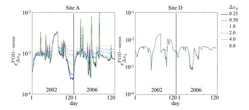
**Fig. 5.** Approximation error at sites A and D for years 2002 and 2006 based on mean-based ROM.
