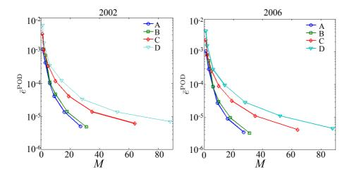
**Fig. 2.** Variation of the mean error,  $\overline{e}^{POD}$ , with respect to number of bases, M, used to construct ROM for year 2002 and 2006 at spatial resolution of 0.25 m.
