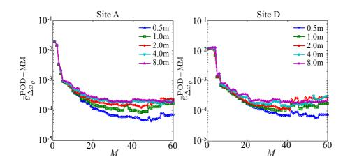
**Fig. 13.** The variation of  $\overline{e}_{\Delta x_g}^{\text{POD-MM}}$ with respect to M for different  $\Delta x_q$  at sites A and D based on the multi-site ROM.
