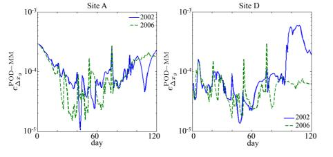
**Fig. 8.** Temporal variations of relative error  $(e_{\Delta x_q}^{\text{POD-MM}})$  in 2002 and 2006 for sites A and D.
