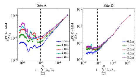
**Fig. 7.** The variation of the POD mapping error  $(\overline{e}_{\Delta x_q}^{\text{POD-MM}})$  with respect to the relative variation not captured by the M number of POD bases to the total variation ( $e_M^{\lambda} = 1 - \sum_{i=1}^{M} \lambda_i / \lambda_T$ ) for different  $\Delta x_q$ . Results are shown for sites A and D for 2006.
