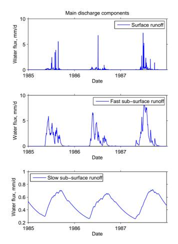
**Fig. 5.** Time series of the streamflow components (direct surface flow, fast subsurface flow and slow (deep) subsurface flow) corresponding to the parameter set of Table 3 and the discharge plot of Fig. 4.
