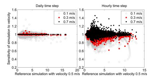
**Fig. 9.** Sensitivity of the discharge simulation with respect to the in-stream flow velocity plotted against the reference simulation with parameters of Table 3 and velocity of  $0.5 \,\mathrm{m\,s}^{-1}$ ; the sensitivity is expressed as the relative difference to the reference simulation for each time step.
