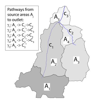
**Fig. 2.** Sketch of the flow paths from a catchment with five source areas  $A_j$  and three channels  $C_j$ . The notation  $C_j^*$  means that the injection into this channel is not concentrated at the upstream end but, in theory, randomized and integrated over the channel length (Bras and Rodriguez-Iturbe, 1985). In practice, we take half of the channel length.
