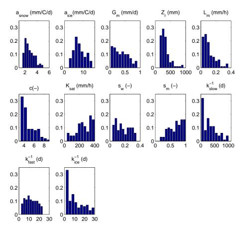
**Fig. 8.** Parameter distributions obtained for the best 100 parameter sets under NSE at a daily time step;  $s_m$ ,  $k_{slow}$  respectively  $a_i$  result from a multiplication of  $s_w$ ,  $k_{fast}$  respectively  $a_s$  with the distribution of the corresponding calibrated scaling parameters.
