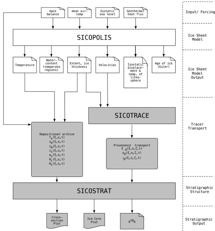
**Fig. 1.** Flow chart of the three programs included in ISOPOLIS: SICOPOLIS – the polythermal ice sheet model. SICOTRACE the tracing program which uses the output from SICOPOLIS and calculates the semi-Lagrangian tracer transport method. SICOSTRAT is the plotting routine for the construct of the stratigraphy.
