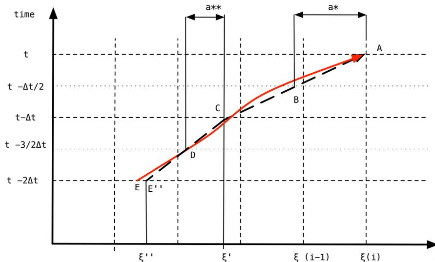
**Fig. 5.** Schematic for the two-step three-time level scheme for one dimension ( $\xi$ ). The red solid curve is the actual trajectory of a particle and the dashed line is the approximation.  $a^*$  is the displacement to the intermediate position where the velocity is evaluated and  $a^{**}$  is the one for the second step.
