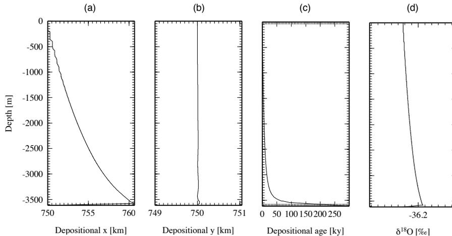
**Fig. 11.** Simulated ice core C1 at  $x = 750$  km,  $y = 750$  km, with **(a)** depositional  $x$  (km), **(b)** depositional  $y$  (km), **(c)** depositional age (kyr), and **(d)**  $\delta^{18}\text{O}$  value.
