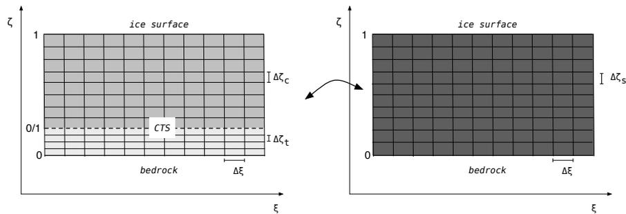
**Fig. 4.** Semi-Lagrangian sigma transformed grid. The original cold and temperate grid on the left are both covered by the semi-Lagrangian grid.
