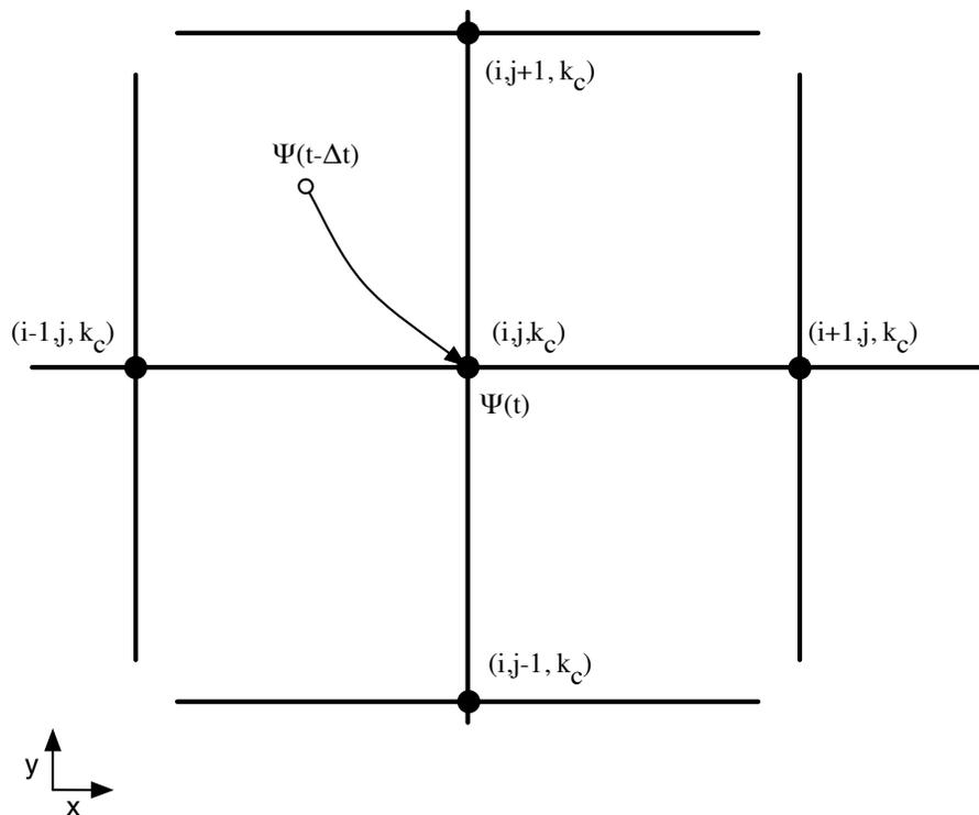
**Fig. 3.** Basic principle of the semi-Lagrangian method explained in the cold ice grid. If the value of  $\Psi(t - \Delta t)$  at the departure point (open circle) is known, the value  $\Psi(t)$  at the desired grid-point  $(i, j, k_c)$  can be calculated. Where  $i$  and  $j$  are the indices of the horizontal grid and  $k_c$  the one for the vertical sigma coordinates in cold ice.
