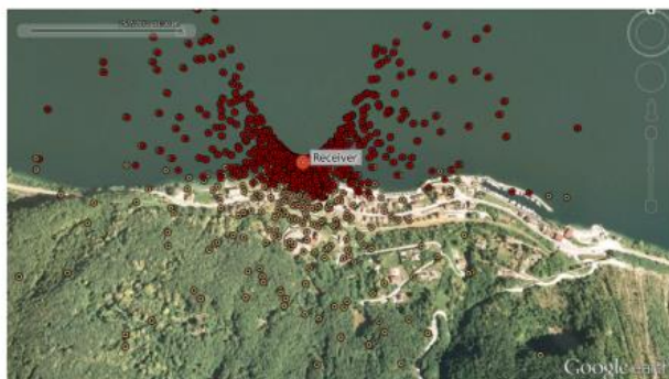
Fig. 15a. Influence of the relief - Specular reflection points on the shore of the Geneva lake (46°24'30N";6°43'6"E).
