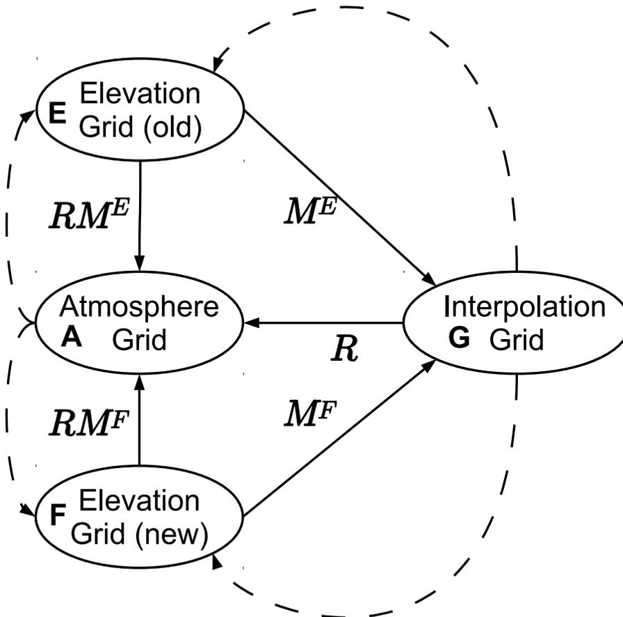
**Fig. 24.** Grid System used to regrid ice surface model state when the elevation grid changes: *E* is the old elevation grid, and *F* is the new one.
