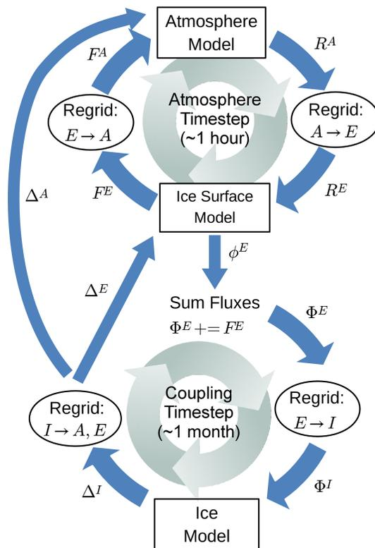
**Fig. 2.** Data flow for the coupling between atmosphere, ice surface and dynamic ice flow models. Outputs from one model are fed as inputs into another. Since the three models run on different grids, regridding is required at each step.
