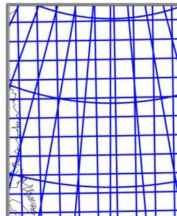
**Fig. 4.** An exchange grid, obtained by overlapping a sample atmosphere grid and ice grid (not to scale). Each resulting grid cell, irregularly shaped, overlaps with exactly one atmosphere grid cell, and exactly one ice grid cell.
