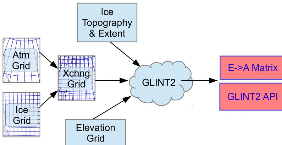
**Fig. 25.** The GLINT2 process flow. GLINT2 produces regridding operations based on a variety of factors: atmosphere and ice grid geometry, ice topography and extent, and elevation levels chosen for the elevation grid.
