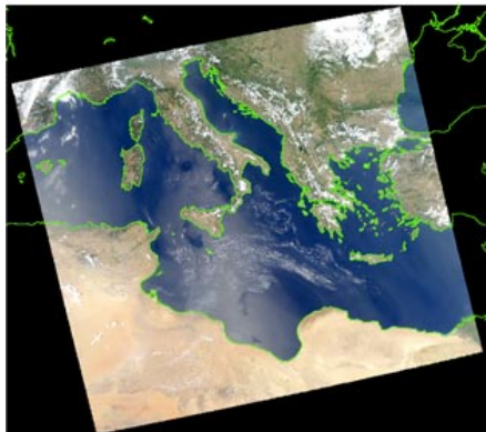
Fig. 1. Equivalent sensor radiance simulation together with an actual MODIS granule that was used as study area. Aqua MODIS granule 2012 day 228 at 12:00 UTC. GEOS-5 temporal fit between 12:00 UT and 18:00 UT, 15 August 2012. RGB (0.67, 0.55, 0.47 \mu\text{m} ).
