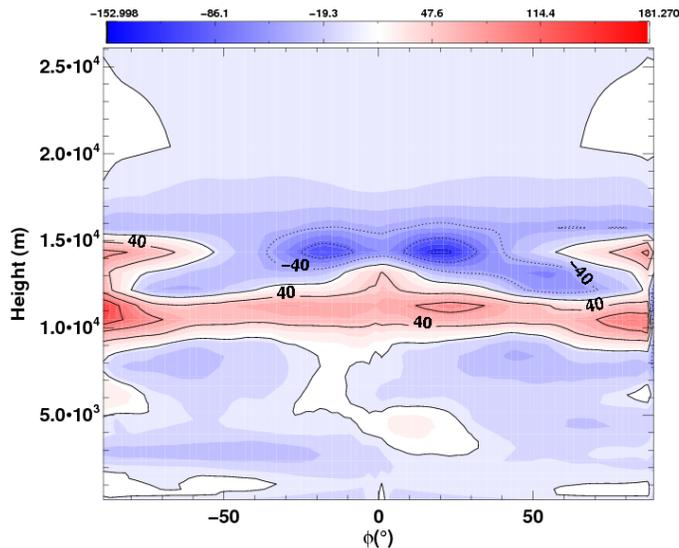
**Fig. 22.** Figure, for the Tidally Locked Earth test (Merlis and Schneider, 2010; Heng et al., 2011b), showing the differences EG-ND of the zonally and temporally averaged EKE (see Table 2 for explanation of model types).
