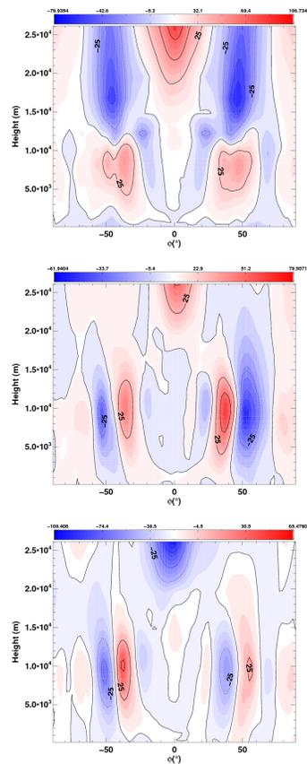
**Fig. 6.** Figure, for the Held–Suarez test (Held and Suarez, 1994), showing the differences EG–ND (top), EG–EG<sub>gc</sub> (middle) and EG–EG<sub>sh</sub> (bottom), of the zonally and temporally averaged EKE. The line contours are the same for all panels (see Table 2 for explanation of model types).
