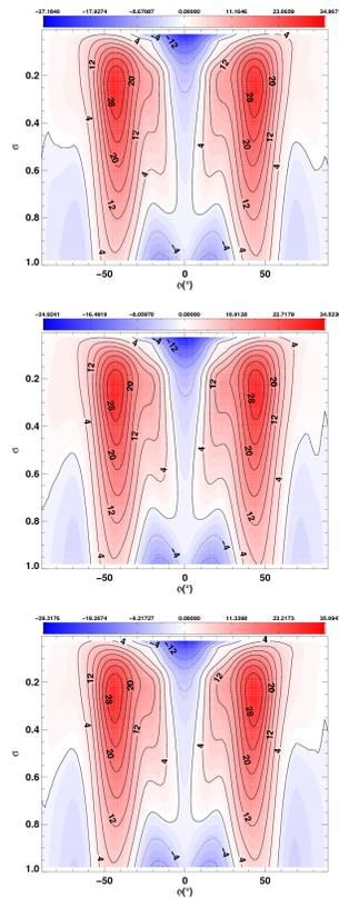
**Fig. 3.** Figure, for the Held–Suarez test (Held and Suarez, 1994), showing the zonally and temporally averaged zonal wind ( $\text{ms}^{-1}$ ) as a function of latitude and  $\sigma$ . Top panel: EG model (also shown in Fig. 2 but reproduced here to aid comparison). Middle panel:  $\text{EG}_{\text{gc}}$  model. Bottom panel:  $\text{EG}_{\text{sh}}$  model (see Table 2 for explanation of model types).
