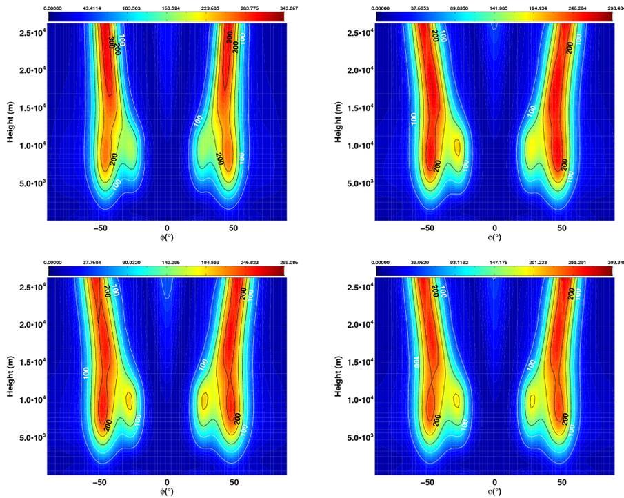
**Fig. 10.** Figure, for the Earth-like test (Menou and Rauscher, 2009), showing the zonally (in geometric height) and temporally averaged Eddy Kinetic Energy (EKE, see Sect. 3.1) as a function of latitude and height. Top left panel: ND, top right panel:  $EG_{sh}$ , bottom left panel:  $EG_{gc}$  and bottom right panel: EG models (see Table 2 for explanation of model types). Note the contours (solid lines) are the same in all plots.
