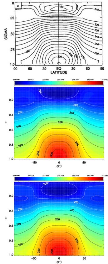
**Fig. 1.** Figure showing, for the Held–Suarez test (Held and Suarez, 1994), the zonally and temporally averaged (i.e. mean from 200 to 1200 days, see Sect. 3.2.1) temperature (K) as a function of latitude and  $\sigma$ . Top panel: original finite difference model Fig. 1 from Held and Suarez (1994), © American Meteorological Society. Used with permission. Middle panel: ND version. Bottom Panel: EG version (see Table 2 for explanation of model types).
