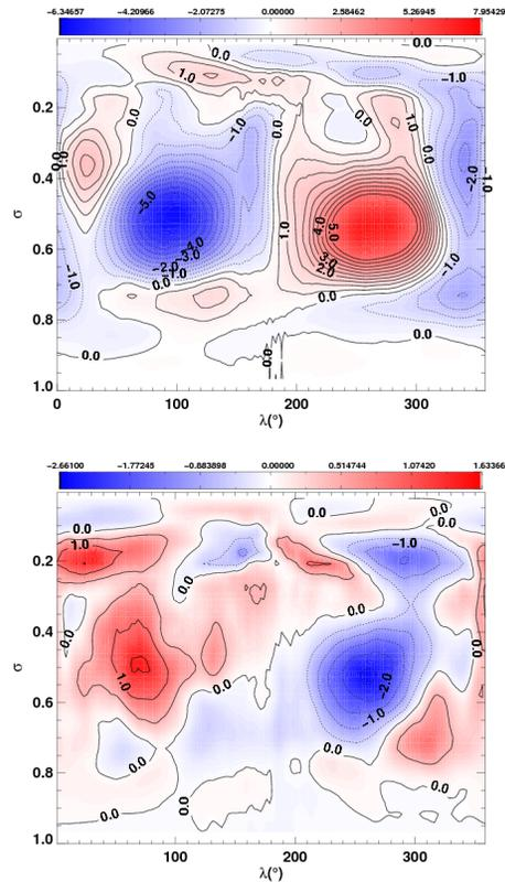
**Fig. 19.** Figure showing, for the Tidally Locked Earth test (Merlis and Schneider, 2010; Heng et al., 2011b), the temporally and meridionally averaged meridional flow for the ND (top panel) and  $EG_{gc}$  (bottom panel) models (see Table 2 for explanation of model types).
