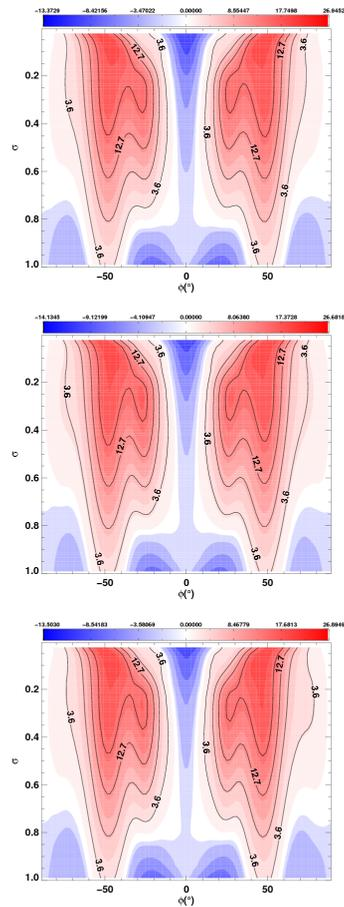
**Fig. 8.** Figures showing, for the Earth-like test (Menou and Rauscher, 2009), the zonally and temporally averaged zonal wind fields for the different EG models. Top panel:, EG, middle panel:, EG<sub>gc</sub> and bottom panel:, EG<sub>sh</sub> (see Table 2 for explanation of model types).
