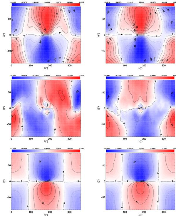
**Fig. 15.** Figure showing, for the Tidally Locked Earth test (Merlis and Schneider, 2010; Heng et al., 2011b), (from the top panels to the bottom panels) the temporally averaged meridional wind at  $\sigma = 0.225$ , 0.525 and 0.975. Results are from the ND (left panels) and EG (right panels) models (see Table 2 for explanation of model types).
