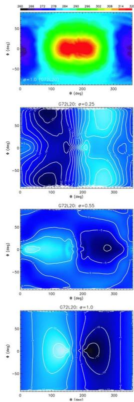
**Fig. 12.** Figure reproduced from Heng et al. (2011b) of the results from the grid-based model of the TLE test case (reproduced by permission of Oxford University Press). Showing (from the top panel to the bottom panel) temperature at 1200 days and  $\sigma = 0.975$ , then, temporally averaged zonal wind at  $\sigma = 0.225$ ,  $0.525$  and  $0.975$ .
