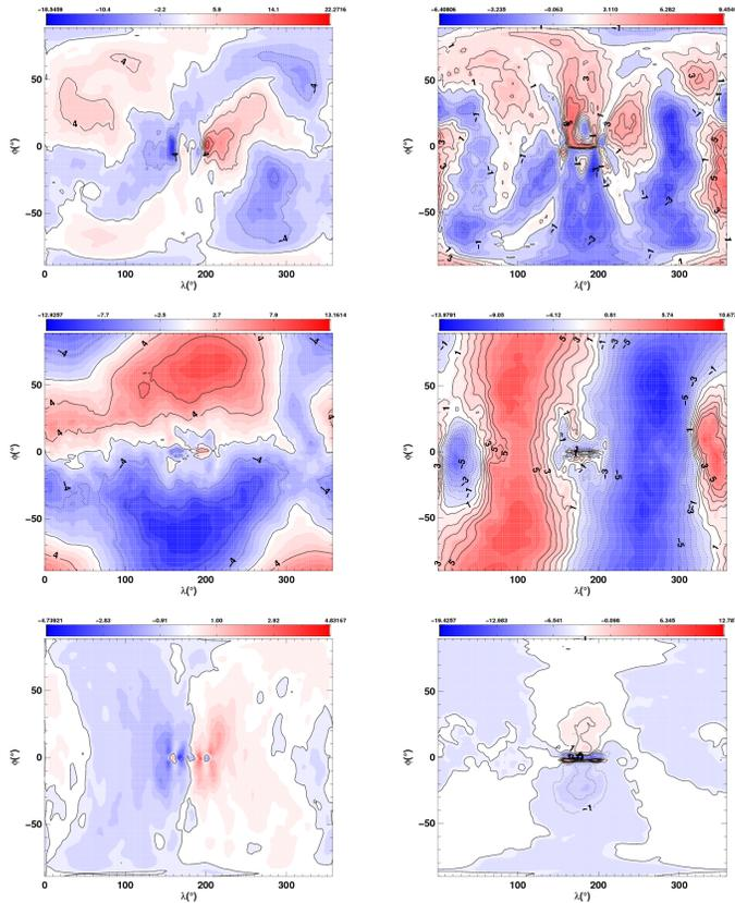
**Fig. 17.** Figure, Tidally Locked Earth test (Merlis and Schneider, 2010; Heng et al., 2011b), showing the differences EG–ND of the temporally averaged, zonal (left panels) and meridional (right panels) winds ( $\text{m s}^{-1}$ ), at  $\sigma = 0.975$ ,  $0.525$ , and  $0.225$ , as the top, middle and bottom rows, respectively (see Table 2 for explanation of model types).
