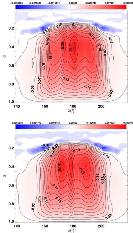
**Fig. 16.** Figure showing, for the Tidally Locked Earth test (Merlis and Schneider, 2010; Heng et al., 2011b), the temporally averaged vertical velocities ( $\text{m s}^{-1}$ ) over the “hot spot” or subsolar point, for the ENDGame dynamical core using the  $\text{EG}_{\text{sh}}$  (top panel) and EG (bottom panel) models (see Table 2 for explanation of model types).
