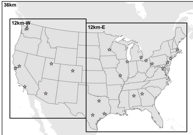
Fig. 3. CAMx North American modeling domain comprised of an outer 36 km resolution grid and two inner, two-way nested, 12 km resolution grids. The 22 cities used for performance evaluation are marked.
