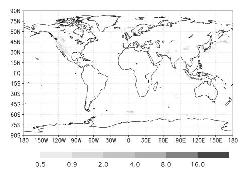
**Fig. 4.** The amplitude of  $2\Delta t$  temperature oscillations on the lowest model level (in Kelvin) after 96 h forecast for the referent model run computed according to Eq. (9).
