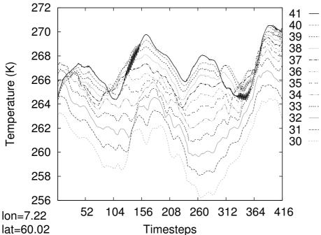
Fig. 5. Temperature (in Kelvin) in one model point on the 12 lowest model levels for each timestep during the 96 h forecast for the referent model run. Level 41 is the lowest model level (full line).
