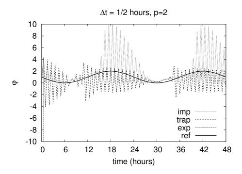
Fig. 1. Numerical solutions of Eq. (1) with implicit (dotted), trapezoid (short dash) and explicit (long dash) schemes for exponent p = 2 and time-step  $\Delta t = 0.5$  h. Function D(t) is also shown (full line) for reference.
