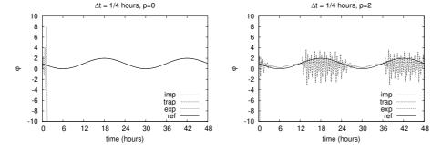
**Fig. 2.** The left figure shows the referent numerical solution of the Eq. (2) for the linear problem with p = 0 and the right figure shows the solution to the non-linear problem with p = 0 and timestep  $\Delta t = 1/4$  h. The results are shown for implicit (dotted), trapezoid (short dash) and explicit (long dash) schemes. Function D(t) is also shown (full line) for reference.
