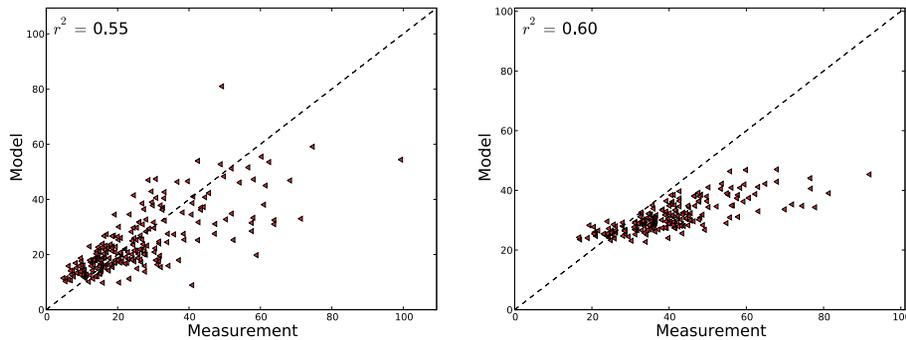
**Fig. 6.** Scatter plot of measured versus Polyphemus using the “rural” option, the GENEMIS temporal profile, a 15 %  $\text{NO}_2$  fraction and stability classes based on Monin–Obukhov length (summer campaign on the left and winter campaign on the right).
