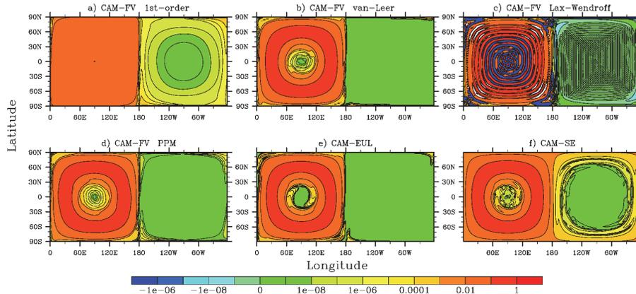
**Fig. 10.** Tracer mixing ratio results for Test 4. At time  $t=T$ , CAM-FV (a) 1st-order, (b) van Leer, (c) Lax-Wendroff, and (d) PPM with the default limiter, (e) CAM-EUL and (f) CAM-SE. The contours use a log scale.
