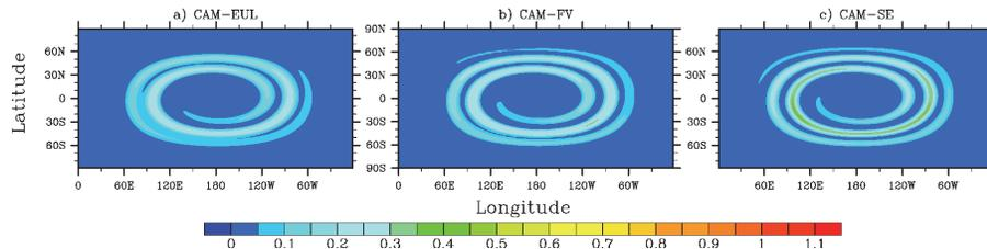
**Fig. 6.** Tracer mixing ratio results using, **(a)** CAM-EUL, **(b)** CAM-FV (PPM) and **(c)** CAM-SE for test 2 at time  $t = T$ . These plots can be compared with the reference solution averaged onto the coarse resolution grid in Fig. 2.
