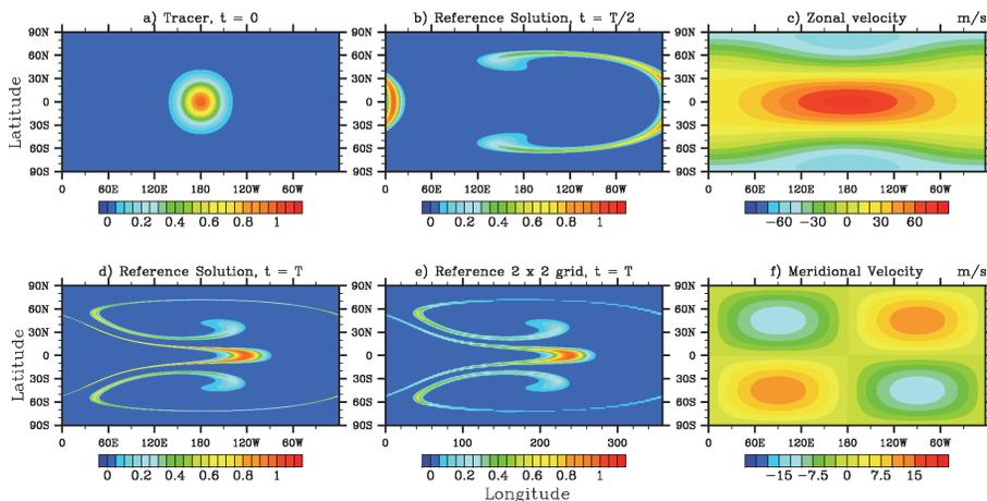
**Fig. 1.** Test 1, **(a)** initial tracer, **(b)** the CAM-FV reference solution at  $t = T/2$  on the  $0.125^\circ \times 0.125^\circ$  grid, **(c)** the zonal velocity  $u$ , **(d)** the reference solution at  $t = T$ , **(e)** the reference solution averaged onto the coarse  $2^\circ \times 2^\circ$  resolution grid at time  $t = T$ , and **(f)** the meridional velocity,  $v$ .
