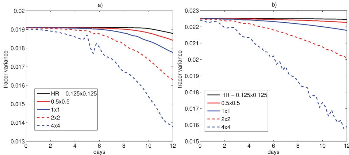
**Fig. 4.** Normalized tracer variance against time for the CAM-FV high resolution (HR) reference solution, and the reference solution averaged onto the coarse grids, for **(a)** test 1, and **(b)** test 2.
