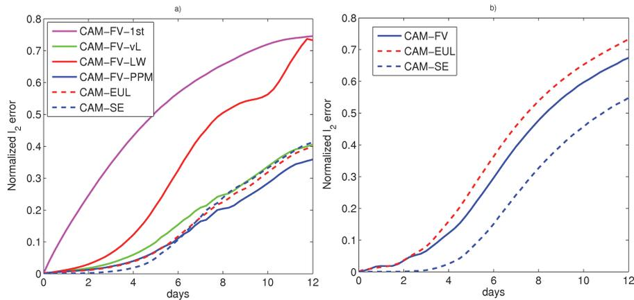
**Fig. 8.** Normalized  $l_2$  error norms against time for **(a)** CAM-FV at  $2^\circ \times 2^\circ$  resolution with the (1st) 1st-order, (vL) van Leer, (LW) Lax-Wendroff, and PPM with the default limiter schemes, CAM-EUL at T85 resolution and CAM-SE for test 1, and for **(b)** the default versions of CAM-FV, CAM-EUL and CAM-SE for test 2.
