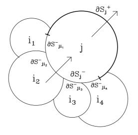
Fig. 1. Schematics for showing the definitions of the boundary segments for the j-th subgrid component.
