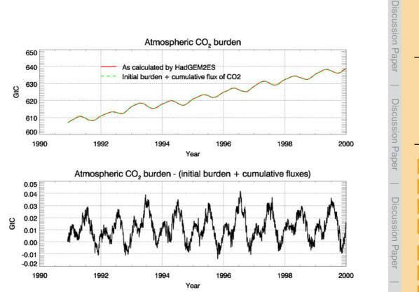
**Fig. 5.** The evolution of atmospheric  $CO_2$  in HadGEM2-ES. Daily atmospheric  $CO_2$  amount (top panel) simulated by HadGEM2-ES (red line), overlaid with the initial atmospheric burden plus the cumulative sum of  $CO_2$  into the atmosphere (dashed green line). The lower panel shows the difference between the two.
