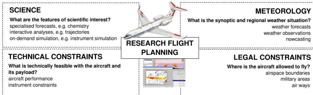
Fig. 1. The major aspects of research flight planning that have to be considered when designing a flight route.
