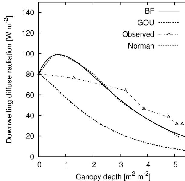
**Fig. 3.** Modeled downwelling diffuse radiation simulated using the BF model (solid line) and GOU model (dashed line). Leaf transmittance  $t = 0.22$  and fraction of diffuse to global radiation  $fDif = 0.17$ . Measured data (open triangles) and model results using the Norman model (dotted) are extracted from Baldocchi et al. (Fig. 5, 1985). Model efficiency,  $ME = 0.46$  and  $-2.45$  for the BF and GOU model, respectively.
