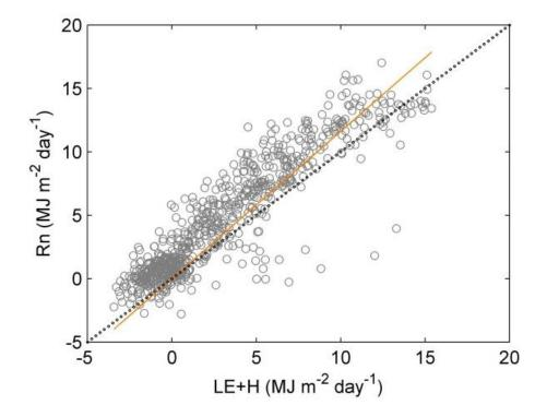
Fig. S2. Comparisons between the observed daily net radiation (Rn) and the sum of daily latent heat (LE) and sensible heat (H) for site of BE-Lon in Belgium (see Fig. S1). The dotted line and orange line is 1:1 line and the linear fit, respectively.
