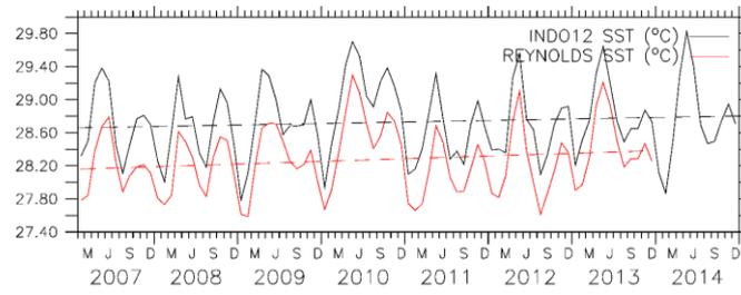
Figure F: Temporal evolution of Sea Surface Temperature over the whole domain (solid line) and associated trend (dashed line), computed from INDO12BIO monthly outputs (black) and from Reynolds satellite product (red).
