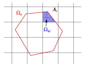
**Figure 5.** Schematic of the notation used to define the overlap between target grid cell  $\Omega_k$  (red polygon) and high-resolution cubed-sphere grid cell  $A_\ell$  (Cartesian-like grid in figure). The overlap area,  $\Omega_{k\ell} = \Omega_k \cap A_\ell$ , is shaded with a cross-hatch pattern in the figure.
