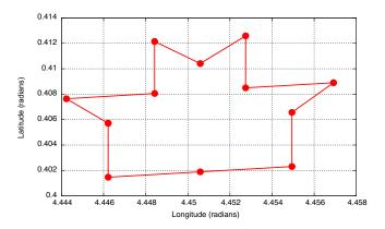
**Figure 4.** An example of a non-convex control volume in variable-resolution CAM-SE. Vertices are filled circles and they are connected with straight lines.
