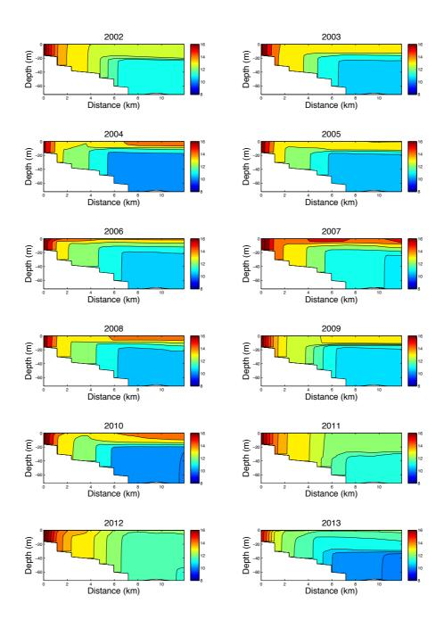
Figure S6. Temperature sections through the tidal mixing front east of Lizard peninsula, along 50.017°N, on day 169 of 2002-13.
