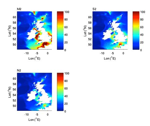
Figure S1. Amplitudes (cm s<sup>-1</sup>) of the M2, S2 and N2 constituents of the local tidal current vector on and around the northwest European shelf (as also used for the configurations around Scotland and in the Western English Channel).
