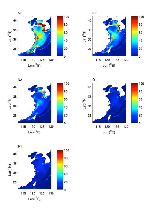
Figure S2. Amplitudes (cm s<sup>-1</sup>) of the M2, S2, N2, O1 and K1 constituents of the local tidal current vector, in the shelf seas around China.
