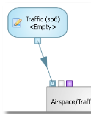
A link between an emitting single terminal and a receiver list terminal
