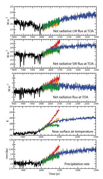
**Fig. 3.** From the top panel and downwards, the figure shows the net global long-wave (positive upwards), short-wave (positive downwards), and total (positive downwards) radiative flux at the top of the atmosphere during the NorESM1-M simulations for 1850 to 2300. The next two panels show diagrams for the global surface air temperature and average daily precipitation. Black: Historic1, green: RCP2.6, blue: RCP4.5, orange: RCP6.0, and red: RCP8.5.
