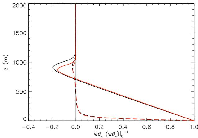
**Fig. 6.** Vertical profile of the total  $\langle \tilde{w}\tilde{\theta}_v + w'\theta'_v \rangle$  (solid line) and subfilter-scale contribution  $\langle w'\theta'_v \rangle$  (dashed) of the virtual potential temperature flux obtained after four hours of simulation by DALES2.0 (black) and DALES 3.2 (red) with the same physical conditions and advection scheme (2nd order central differences).
