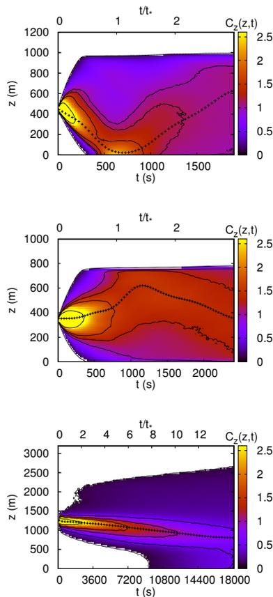
**Fig. 14.** Evolution on time of the vertical concentration (crosswind integrated) of a plume released as a function of the releasing time (dimensional and non-dimensional) for (top) dry convective conditions, (middle) stratocumulus topped boundary layer, and (bottom) shallow cumulus topped boundary layer. Concentration has been multiplied by a factor 1000 to obtain a convenient scale. The crosses indicate the position of the maximum concentration.
