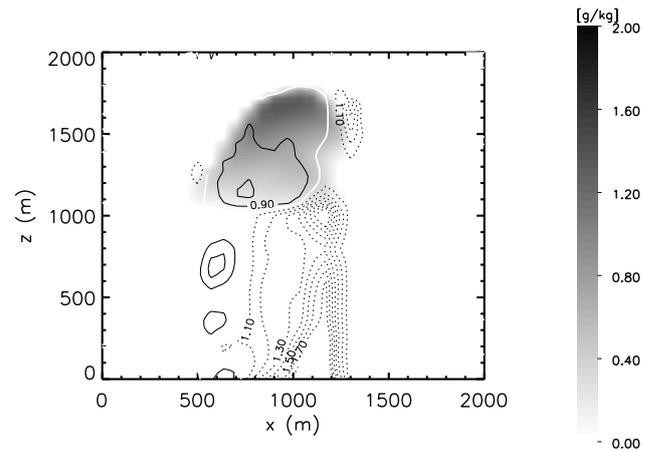
**Fig. 15.** Instantaneous vertical cross section of the cloud water  $q_c$  ( $\text{g/kg}$ ) content and the photostationary state ( $\Phi$ ) calculated using the  $\text{NO}$ ,  $\text{NO}_2$  and  $\text{O}_3$  mixing ratios. At chemical equilibrium  $\Phi = 1$ .
