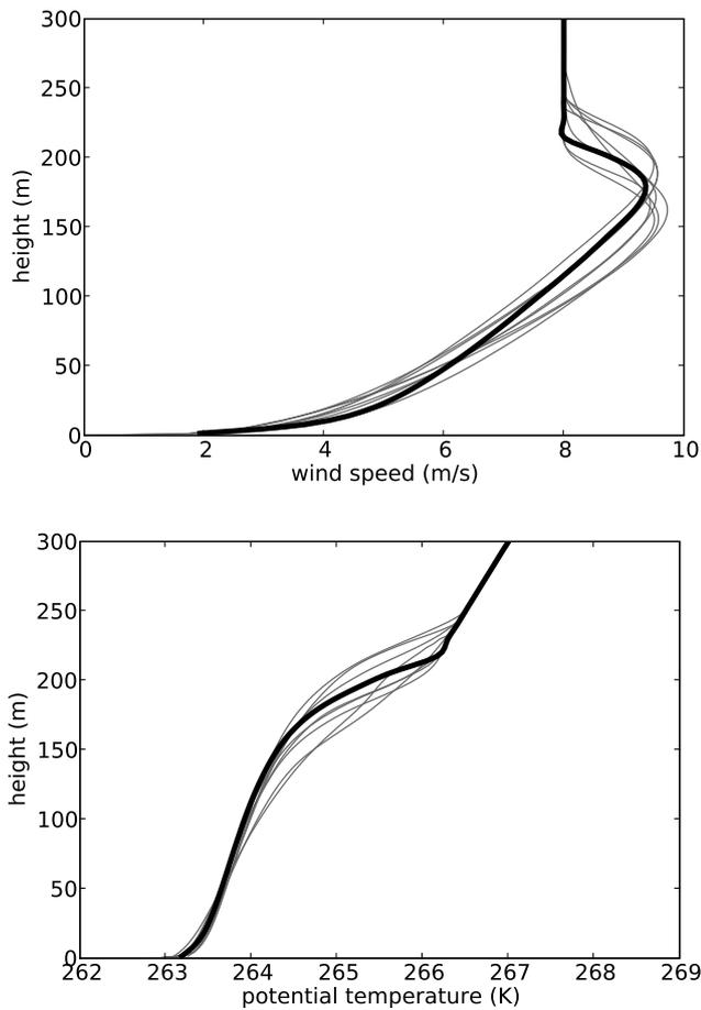
**Fig. 8.** Profiles of mean wind speed (top) and potential temperature (bottom) for the first GABLS1 LES intercomparison (average over 9th hour of simulation). Solid black line: DALES result at 3.125 m resolution and  $c_f = 2.0$ ; grey lines: results of other participants at 3.125 m resolution.
