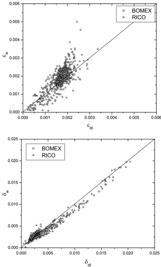
**Fig. 11.** Comparison of LES derived fractional entrainment and detrainment rates  $\epsilon_q$  and  $\delta_q$  using  $\phi = q_t$  based on Eq. (110) (horizontal axis) versus LES estimates of these rates  $\epsilon_w$  and  $\delta_w$  based on the vertical velocity equation (Eqs. 111 and 112).
