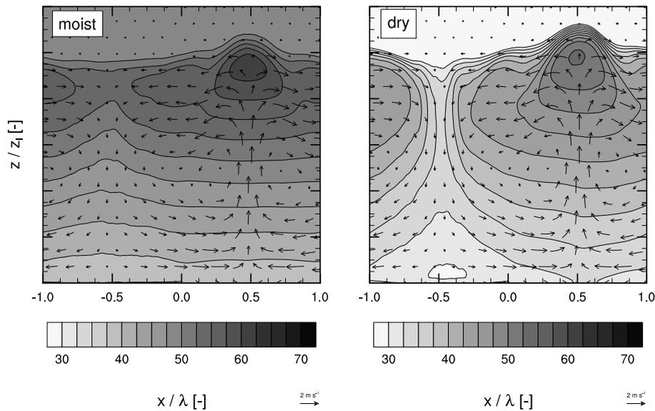
**Fig. 12.** Cross section of the 1-h-averaged relative humidity  $\overline{RH}$  for a case with a moist free troposphere (left) and a case with a dry free troposphere (right). The horizontal coordinates are scaled by the patch size  $\lambda$  and the vertical coordinates are scaled by the CBL height  $z_1$ . Vectors indicate the wind direction and magnitude. From van Heerwaarden and Vilà-Guerau de Arellano (2008).
