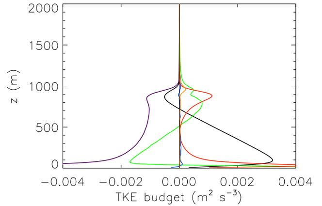
**Fig. 4.** Vertical profile of the various terms of the TKE budget in a sheared CBL: total tendency (orange), buoyancy (black), dissipation (violet), transport and pressure (green), shear (red), and the residual (blue).
