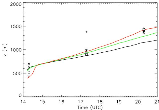
**Fig. 7.** Boundary layer height  $z_i$  observed by radiosondes launched at different facilities of ARM campaign (symbols) and obtained by means of LES: without shear (black), including a constant geostrophic wind of  $10 \text{ ms}^{-1}$  in the east-west direction (green), and prescribing the observed mean wind (red). Adapted from Pino et al. (2003).
