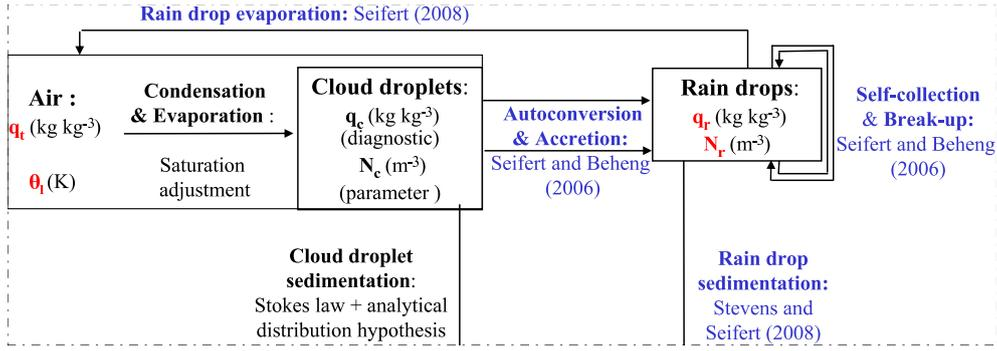
**Fig. 3.** Representation of the prognostic thermodynamical variables  $\tilde{\theta}_1$ ,  $\tilde{q}_t$ , the microphysical parameter and variables  $N_c$ ,  $q_c$ ,  $\tilde{N}_r$ ,  $\tilde{q}_r$ , and the microphysical processes relating these variables.
