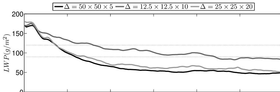
**Fig. 17.** The liquid water path for DYCOMS2 using the 5th order advection scheme for various resolutions. Runs are performed without  $\chi^*$ -correction, which in itself significantly enhances the LWP.
