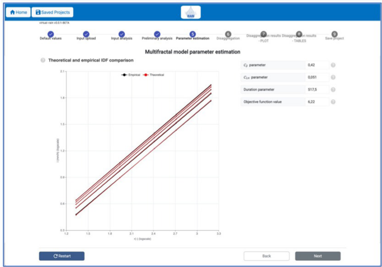
Figure A11. MRC calibration interface showing the comparison between imposed and calibrated IDF curves for the selected return periods, together with the estimated MRC parameters and objective-function value.
