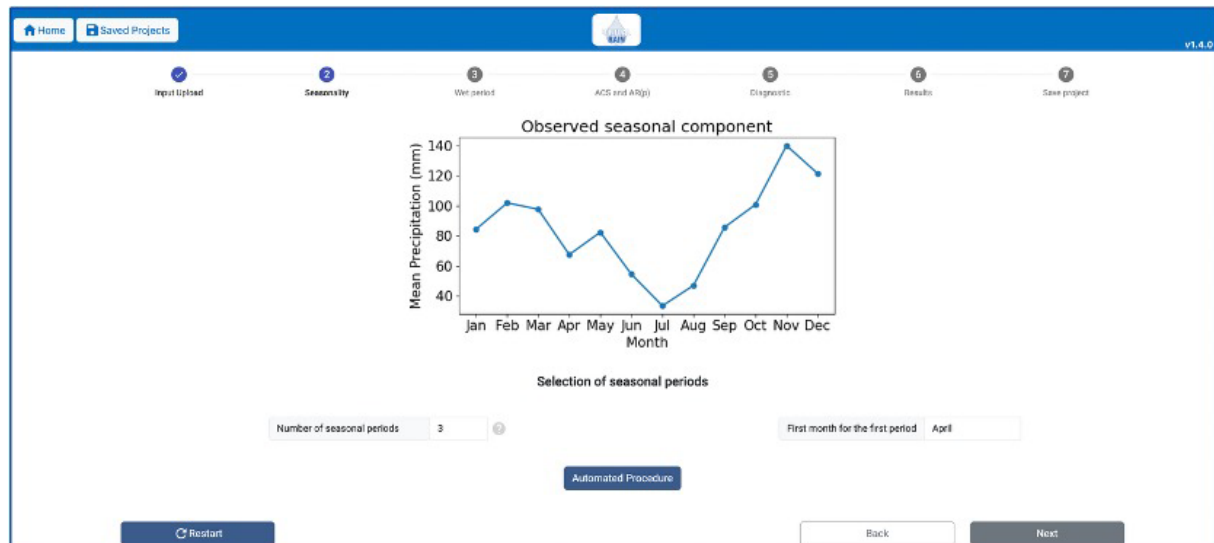
Figure A3. Seasonality interface supporting the user-defined selection of the number of seasonal periods and the starting month. The seasonal partition is specified by the user and is not automatically determined by the software.
