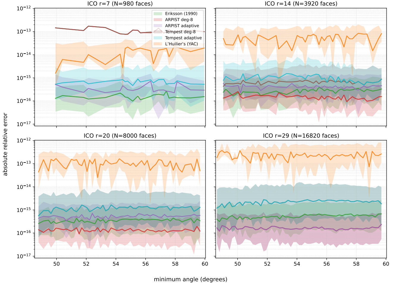
Figure S5. Four-panel polygon plots for icosahedral meshes at resolutions r \in \{7, 14, 20, 29\} . Shaded bands show the 5%–95% envelope within each minimum-angle bin; the center line is the bin-wise mean (computed in \log_{10} -error space). Angles are grouped into 60 log-spaced bins over the observed minimum-angle range. (60 balances resolution with per-bin sample size across all meshes)
