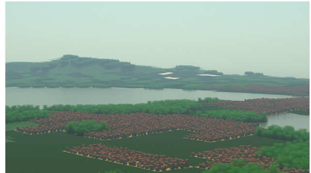
Figure 5. RGB view of a synthetic scene created after the area of Mbita, on Lake Victoria in Kenya. The surface shape (a triangulation of the Copernicus GLO-30 DEM) is assigned different reflection models (e.g. water, diffuse, RPV) based on land cover information contained in a texture encoded as a PNG image. Where relevant, land areas are also tiled with 3D objects at a reduced memory cost using instancing: a few templates (e.g. village, forest) are cloned many times to create a radiatively plausible reflection pattern. See also Sect. 8.2.3 for a similar example.
