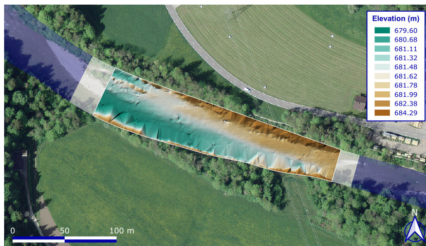
Figure A3. High-resolution (25 cm) riverbed DEM used to define the 3D meshes of the test case (background image from © Google Maps 2024).
