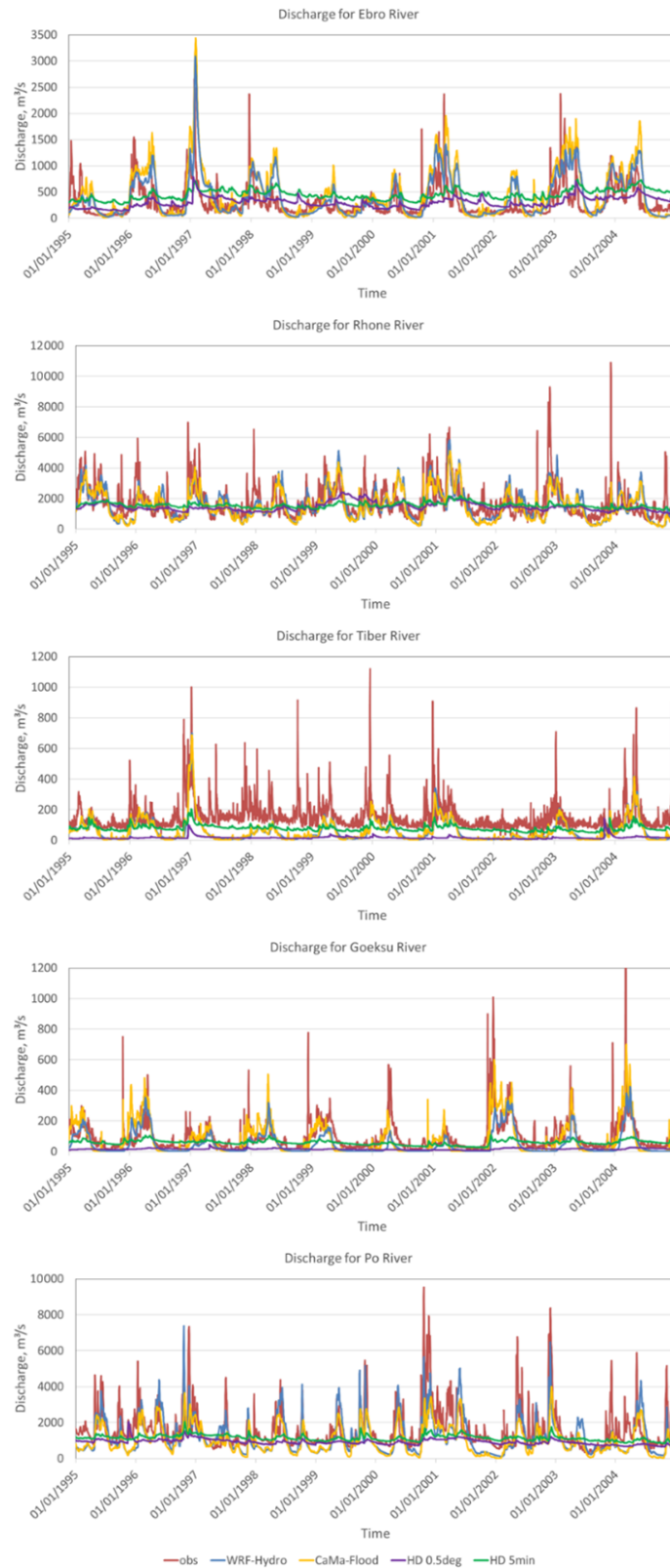
Figure 2. Observed and simulated daily discharge for the Ebro, Rhone, Tiber, Goeksu and Po rivers for common 10 years from 1995 to 2004. Simulations include ENEA-REG-driven WRF-Hydro and CaMa-Flood, as well as the HD model at 0.5° and 5 min spatial resolutions, evaluated near the corresponding gauge stations.
