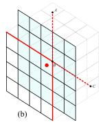
Figure 2. (a) Adjacent area of panels 1, 4 and 5. (b)  $5 \times 5$  reconstruction stencil nearby panel corner is represented by shade. The cell contains red dot is the target cell on panel 4; the magenta points are overlapped GQPs shared by panel 1 and panel 5; red solid lines are boundary of panel 4, red dash lines are extension line of panel 4 boundary line. A and C are points on dash line, B is the upper right corner point of panel 4.
