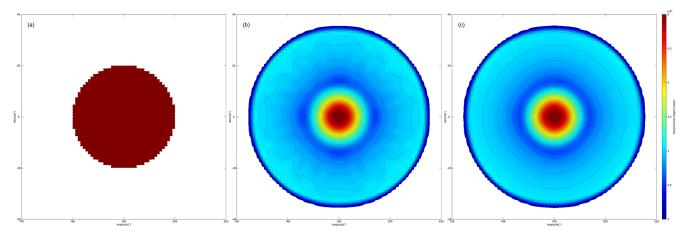
**Figure 18.** Geopotential of dam-break test case on C90 grid at 2nd hour. (a) Initial condition, (b) WENO 1D, (c) WENO 2D. The horizontal resolution for both schemes is C90. Shaded and contour from  $3.2 \times 10^4$  to  $6 \times 10^4$  m, with contour interval  $10^3$  m.
