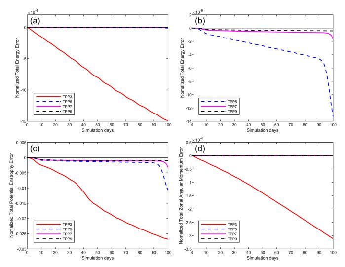
**Figure 14.** Time series of normalized conservation errors for the Rossby–Haurwitz wave simulation on the C90 grid over days 0 to 100, with LMARS scheme as Riemann solver. (a) Normalized total energy error for TPP3, TPP5, TPP7 and TPP9. (b) The total energy normalized error for TPP5, TPP7 and TPP9. (c) Normalized potential enstrophy error for TPP3, TPP5, TPP7 and TPP9. (d) Normalized total zonal angular momentum error for TPP3, TPP5, TPP7 and TPP9.
