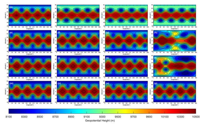
**Figure 15.** Geopotential of Rossby–Haurwitz wave on C90 grid, the rows represent the spatial reconstruction scheme with TPP3, TPP5, TPP7 and TPP9 the columns stand for simulation day 30, 60, 90 and 100. Contours from 8100 to 10 500 m with interval 200 m.
