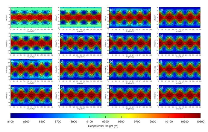
**Figure 16.** Geopotential of Rossby–Haurwitz wave at simulation day 80. The rows represent spatial reconstruction with TPP3, TPP5, TPP7 and TPP9. The columns stand for grid C45, C90, C180 and C360. Contours from 8100 to 10 500 m with interval 200 m.
