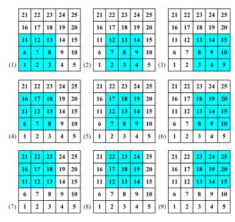
**Figure 6.** Stencils of 5th order WENO 2D. The high order stencil contains cells No. 1–25, blue ones represent the cells in substencils (1)–(9).
