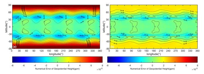
**Figure 10.** Numerical errors (simulation result minus exact solution) of geopotential for steady state flow with Riemann solvers (a) LMARS and (b) AUSM<sup>+</sup>-up. The reconstruction scheme is TPP5, and the model resolution is C90.
