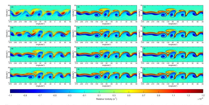
**Figure 17.** Relative vorticity of perturbed jet flow. (a)–(c) represent the results of TPP5 scheme with resolutions C45, C90, C180. (d)–(f) represent the results of TPP7 scheme with resolutions C45, C90, C180. (g)–(i) represent the results of TPP9 scheme with resolutions C45, C90, C180. (j)–(l) represent the results of TPP11 scheme with resolutions C45, C90, C180.
