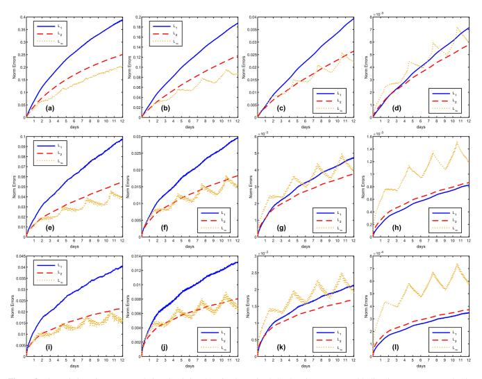
Figure 8. The variation of norm errors during simulation days for the cosine bell advection test case, with direction parameter  $\alpha = 0$ . The rows represent reconstruction schemes TPP3, TPP5 and TPP7, the columns stand for grid C30, C45, C90 and C180.
