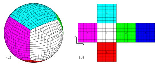
Figure 1. Cubed sphere grid. (a) Physical space; (b) computational space. Six panels are identified by indices from 1 to 6.
