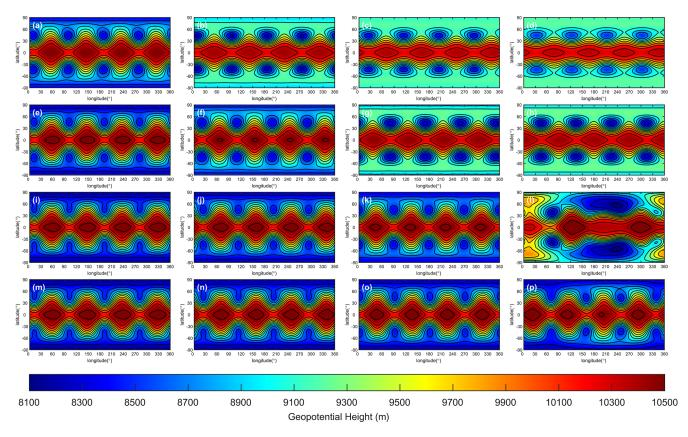
Figure 13. Geopotential of Rossby–Haurwitz wave simulated by TPP3 scheme. The rows represent grid C45, C90, C180 and C360, the columns stand for simulation day 14, 30, 60, 90. Contours from 8100 to 10 500 m with interval 200 m.
