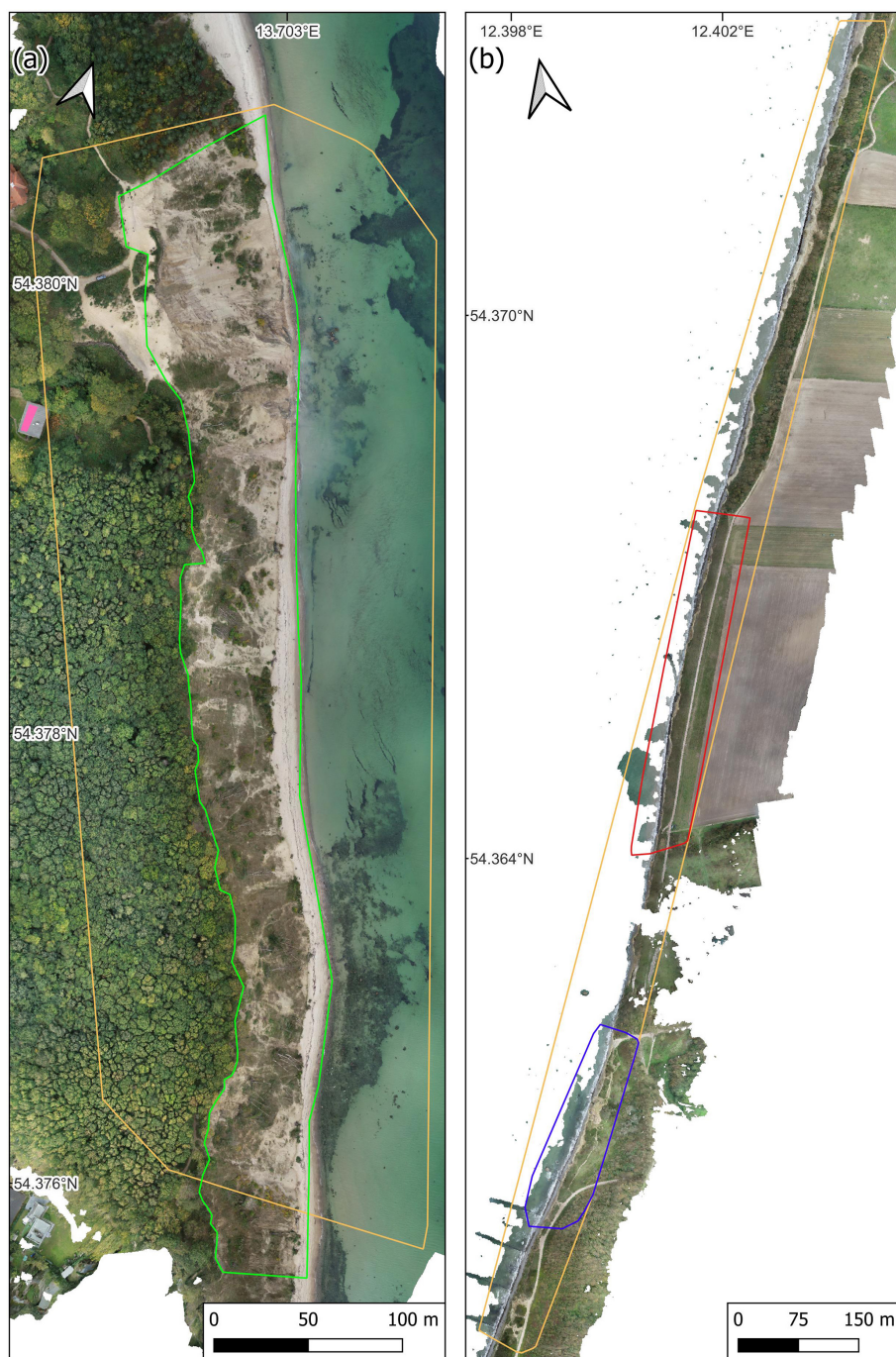
Figure 4. Orthophotos based on images from Field Campaign 6 with stable feature (pink filled polygon), sand cliff (green polygon), bunker area (blue polygon), coastal erosion area (red polygon), and the minimum bounding box (yellow polygons) of all images taken automatically on that day. (a) Sellin; (b) Wustrow.
