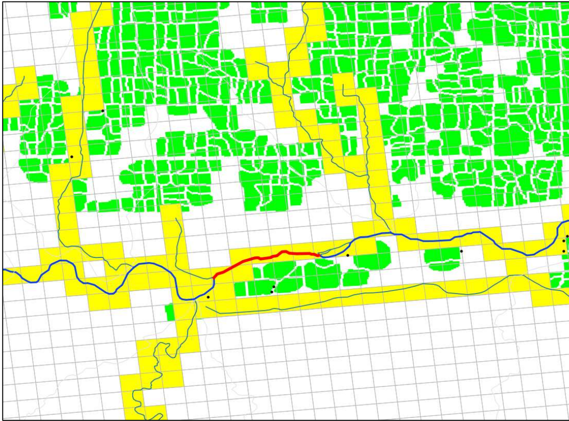
Figure S6. MODFLOW grid cells (yellow) in connection with SWAT+ channels.
