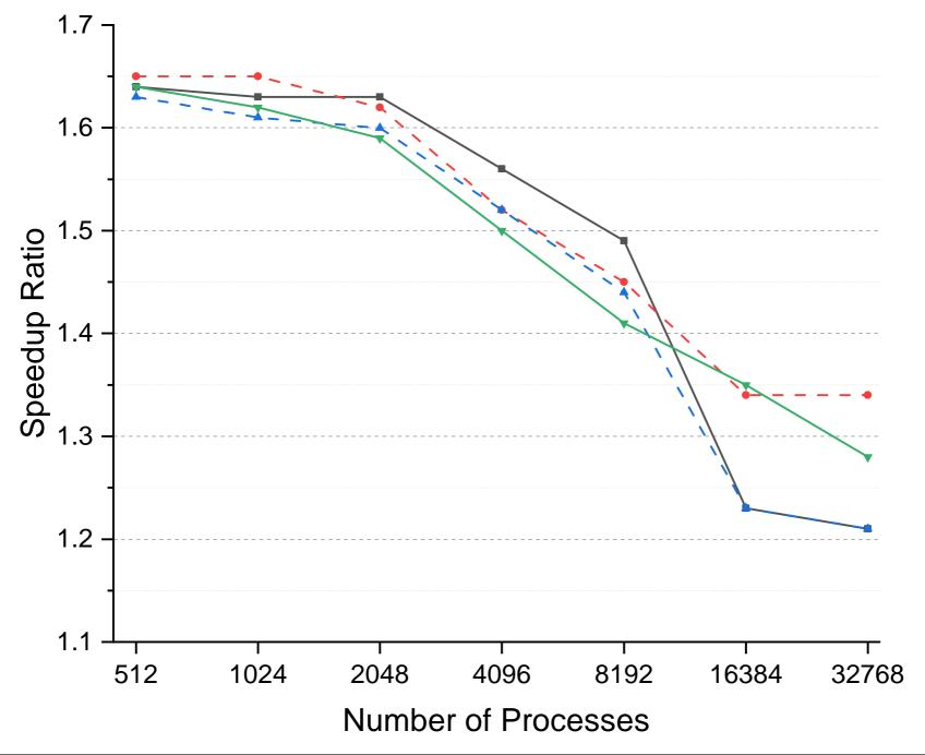
Maximum runtime speedup of the FVWAM between the graph communication topology without reordered processes and the point-to-point communication
