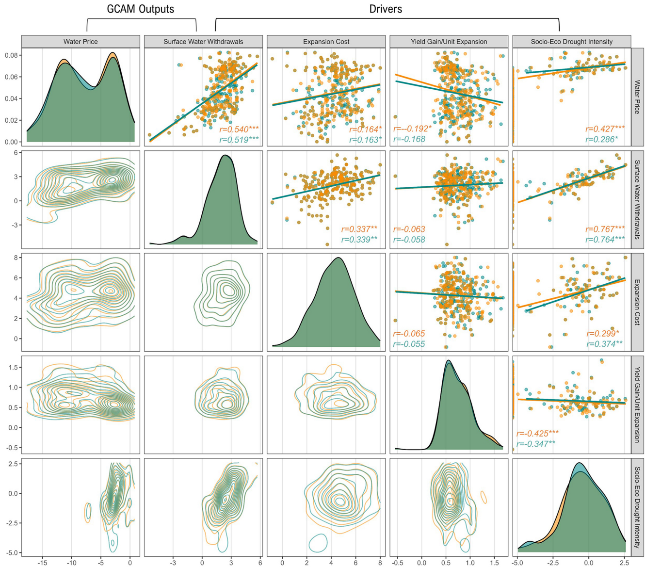
Figure 11. Paired density plots (lower half) and Pearson correlation plots (upper half) among drivers and GCAM outputs in 2050 under Feedbacks and No Feedbacks scenarios for selected basins. Drivers include the cost for incremental expansion storage, median water gain per unit storage capacity expansion at GCAM solved supply level, and socioeconomic drought intensity. GCAM outputs include water prices and water withdrawals (or demands). The orange and blue colors denote Feedback and No Feedback scenarios, respectively. The asterisks indicate the level of correlation (e.g., three asterisks mean strong correlation). Basins are included for the linear regression for water gain per unit expansion and socioeconomic drought intensity if the water supply is above the maximum natural yield and there is a deficit between sub-annual demand and natural runoff. The maximum natural yield is the amount of natural water that can be provided without any reservoir regulation. All variables are normalized with log transformation, and both axes are unitless.
