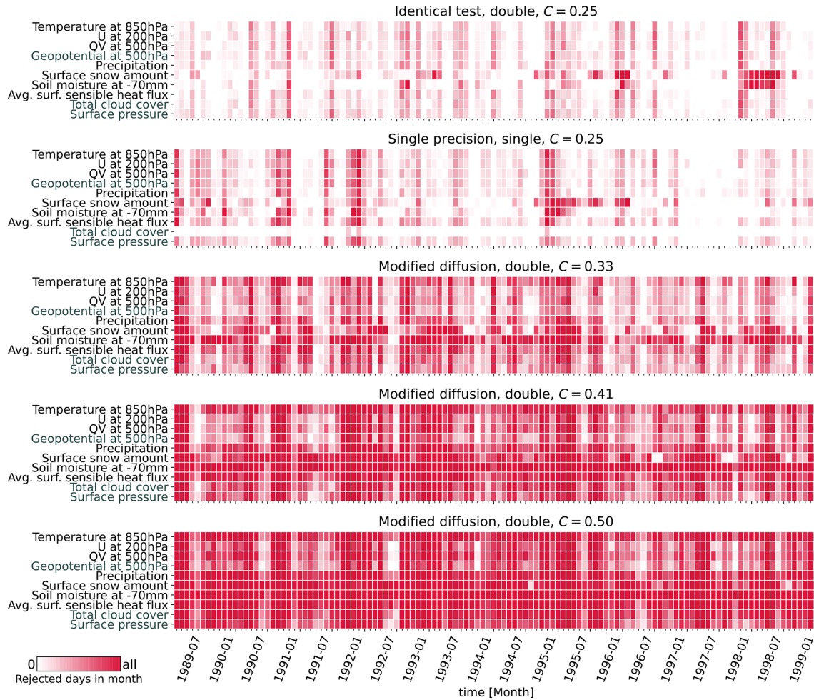
Figure 2. Monthly averaged test decisions for all five test ensembles and a representative subset of 10 variables out of 47. Variables in black are output daily, while those in gray are output 12-hourly.
