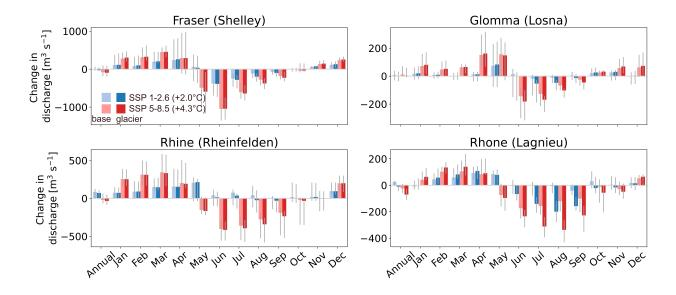
Figure S13: Absolute change in mean annual and mean monthly discharge at the upstream stations for the period 2070–2099 compared to 1990–2019 for  $\text{CWatM}_{\text{base}}$  and  $\text{CWatM}_{\text{glacier}}$ , shown per SSP scenario which translate into warming levels of +1.9°C and +4.2°C compared to pre-industrial time. The height of the bar indicates median change of GCMs and the grey lines indicate the maximum and minimum change of GCMs.
