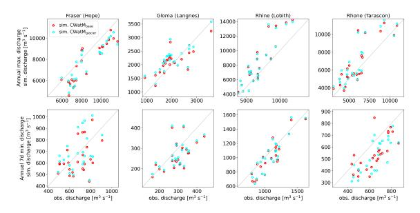
Figure S7: Simulated against observed annual minimum and maximum discharge of the 30 years in the past (1990–2019). The different colours refer to  $CWatM_{base}$  and  $CWatM_{glacier}$ .
