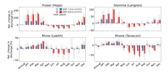
Figure S12: Relative change in mean annual and mean monthly discharge at the downstream stations for the period 2070–2099 compared to 1990–2019 for  $CWatM_{base}$  and  $CWatM_{glacier}$ , shown per SSP scenario which translate into warming levels of +1.9°C and +4.2°C compared to pre-industrial time. The height of the bar indicates median change of GCMs and the grey lines indicate the maximum and minimum change of GCMs.
