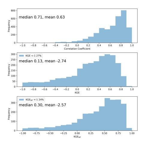
Figure S9: Histograms of performance of six global parameter sets: Correlation coefficient, KGE and the non-parametric version of the KGE (KGE<sub>NP</sub>) of monthly discharge. The mean and median values are annotated as well as the percentage of gauges with KGE and KGE<sub>NP</sub> below -1.
