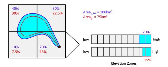
Figure S1: Schematization of the area reduction approach for a glacier that covers multiple grid cells used in this study. The same relative area reduction is applied to all grid cells that the glacier covers. In each grid cell, the glacier covered area is omitted in CWatM as shown on the right hand side. The black dot on the left hand side indicates the terminus of the glacier and therefore the grid cell to which glacier-sourced melt of the entire glacier is routed.
