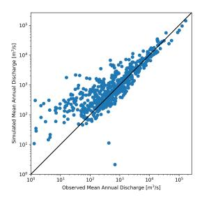
Figure S10: Simulated compared to observed mean annual discharge at gauges used for calibration for the time period 1990–2019. The ensemble mean of simulations with six parameter sets is used.
