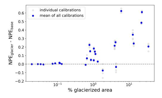
Figure S20: The performance difference between  $\mathrm{CWatM}_{\mathrm{glacier}}$  and  $\mathrm{CWatM}_{\mathrm{base}}$  compared to the glacier coverage. The data is the same as for Fig. 7. Results are shown for individual calibrations (grey dots) and mean of all calibrations (blue dots) for the 10 year period 2004 to 2013.
