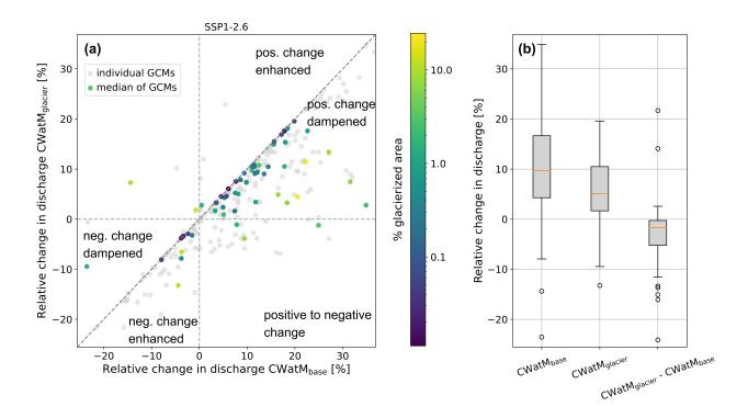
Figure S22: Comparison of relative future change for annual discharge at end of the  $21^{\rm st}$  century for CWatM<sub>base</sub> and CWatM<sub>glacier</sub> for 56 glacierized river basins for SSP1-2.6. (a) Colored dots show the median of all GCMs and grey dots show individual GCMs. (b) Boxplots showing the relative future change of all basins for CWatM<sub>base</sub> and CWatM<sub>glacier</sub> and their difference.
