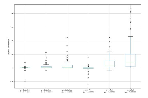
Figure S24: Boxplots of difference in precipitation and snowfall input across the 56 glacierized river basins between  $\text{CWatM}_{\text{glacier}}$  with different precipitation factors  $(p_f)$  and  $\text{CWatM}_{\text{base}}$  (base) for annual averages for the period 1990–2019. Each boxplot is based on 56 data points.
