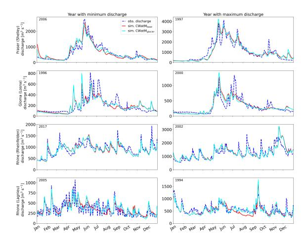
Figure S6: Hydrographs of the year with minimum and maximum annual discharge sum for the upstream stations of the study basins. For the Rhone, the year with the second smallest discharge was chosen as the minimum year, because for the year with the lowest discharge, no observational data was available.
