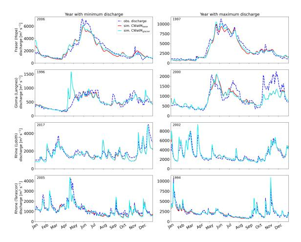
Figure S5: Hydrographs of the year with minimum and maximum annual discharge sum during the 30-year period 1990–2019 for the downstream stations of the study basins. Years 2000 or later fall within the calibration period. For the Rhone, the year with the second smallest discharge was chosen as the minimum year, because for the year with the lowest discharge, no observational data was available.
