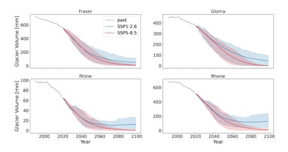
Figure S14: Glacier volumes for the selected rivers simulated with OGGM, shown as water equivalent per total river basin area [mm], per SSP scenario which translate into mean warming levels of +1.9°C and +4.2°C compared to pre-industrial time. Shaded area shows the total range of the five GCMs.
