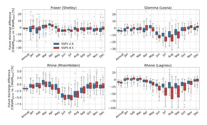
Figure S11: Relative difference in mean annual and mean monthly discharge of  $CWatM_{glacier}$  compared to  $CWatM_{base}$  at the upstream gauges for 30 years from 2070–2099, shown per SSP scenario which translate into warming levels of  $+1.9^{\circ}C$  and  $+4.2^{\circ}C$  compared to pre-industrial time.
