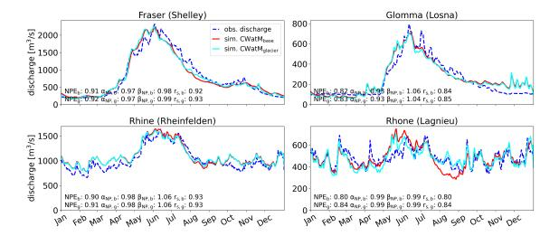
Figure S4: Mean hydrographs of the evaluation period (1990–1999) for the upstream station of the study basins. As insert the NPE and its error components over the whole evaluation period are given for CWatM<sub>base</sub> (index b) and CWatM<sub>glacier</sub> (index g) ( $\alpha_{NP}$ : variability,  $\beta_{NP}$ : mean,  $r_s$ : dynamics; Pool et al., 2018). Values closer to 1 indicate a better match.
