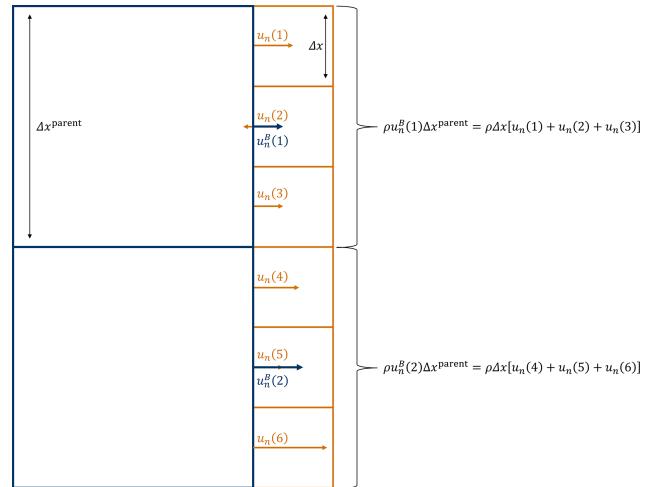
Figure 1. A 2D illustration of a nested setup in which the integration length scales are set to the grid size of the parent model. In this setup, the mass flux through a parent cell (blue) at the boundary of the child model (brown) is conserved, while the child model is free to generate turbulence on smaller scales.
