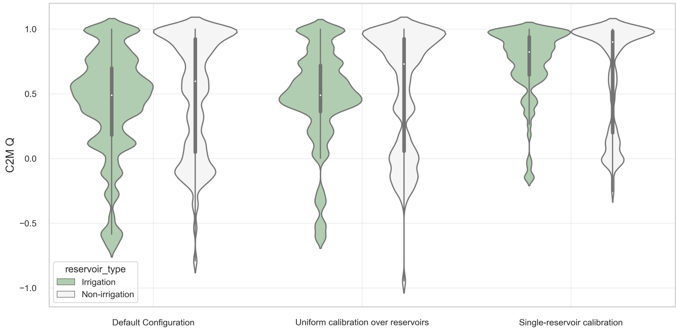
Figure S2. Distribution of the reservoir model performance index C_{2M} over outflows before and after calibration in irrigation (green) and non-irrigation reservoirs (light grey). The default configuration stands for the default setting of the model, the two others are respectively the model calibration performed uniformly on all reservoirs and on each reservoir individually.
