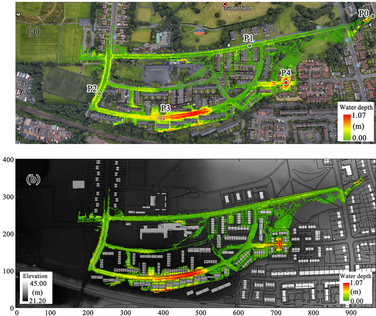
Figure 7. Flood inundation extent at t = 4200 s calculated by (a) the dg2 solver and (b) the improved SGC solver. Background maps in (a) are © Google Maps screenshots.
