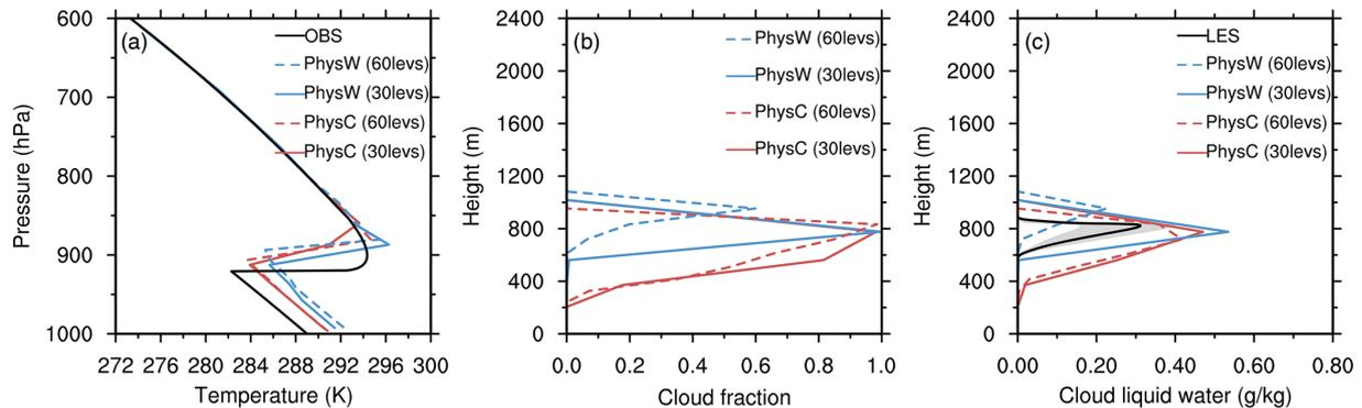
**Figure 15.** Time-averaged (a) temperature (units: K), (b) cloud fraction, and (c) cloud liquid water mixing ratio (units:  $\text{g kg}^{-1}$ ) simulated by PhysC (red) and PhysW (blue) for DYCOMS-RF01. The solid lines show the model runs with 30 full layers (30levs), and the dashed lines show that using 60 layers (60levs). The black solid line in (a) shows the observation from IOP data. The black solid line in (c) shows the LES ensemble mean, and the gray shading represents its spread.
