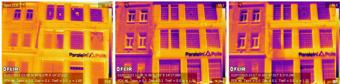
Figure S15: Three infrared snapshots from observation location 6 — view of south facing wall from 3 July 2015 01:08 UTC (03:08 local time), 10:08 UTC (12:08 local time) and 13:17 UTC (15:17 local time).
